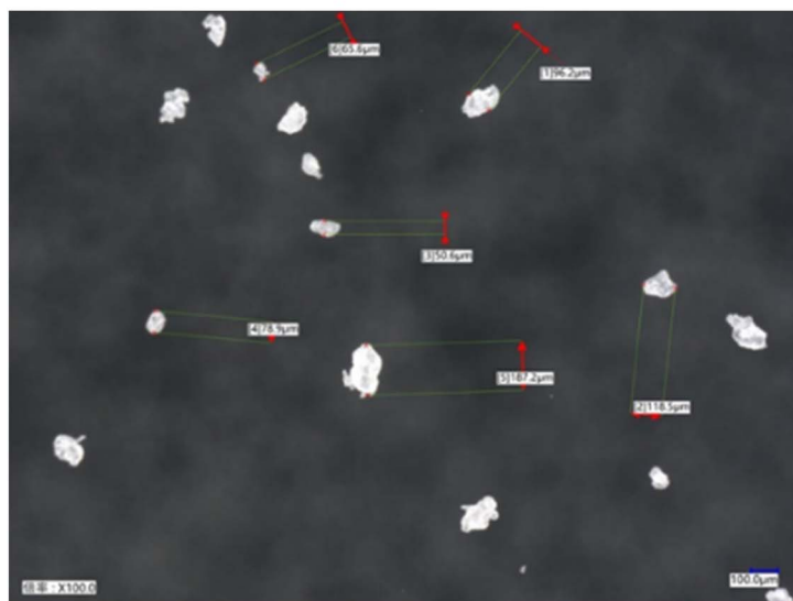
Fig. 37 Biomass biodegradable resin powder. (Top left) PLA base, (Top middle) starch base and (Top right) cellulose base. Optical microscopic observation of PLA-based 100% biomass biodegradable resin powder (Below).
