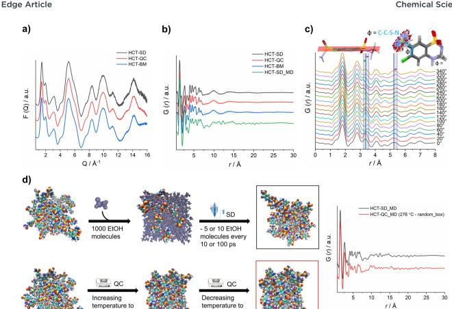
Fig. 4 (a) F(Q) and (b) PDF of experimental HCT polyamorphs and simulated QC method (green curve) with an offset in the y-axis for better clarity; (c) simulated PDF of HCT single molecule when varying the dihedral angle  $\Phi$ ; and (d) schematic representation of the MD simulations of both SD and QC methods with the corresponding simulated PDF curves in black and red, respectively (offset in the y-axis for better clarity). EtOH stands for ethanol.
