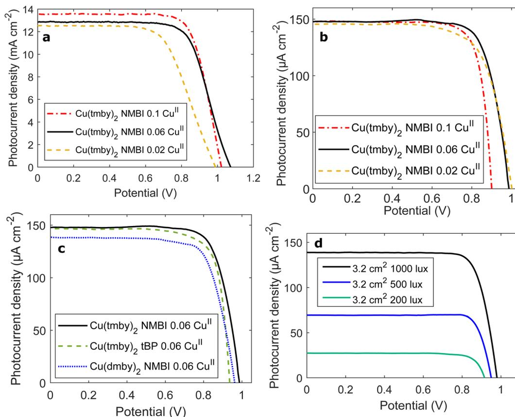
**Fig. 4** *J*-*V* sweeps of XY1:L1-sensitised photovoltaic cells (a) 0.384 cm<sup>2</sup> cells by electrolyte composition at one-sun AM 1.5G irradiation. (b) and (c) 0.384 cm<sup>2</sup> cells by electrolyte composition at 1000 lux ambient illumination (fluorescent lamp). (d) 3.2 cm<sup>2</sup> cells by illumination level.
