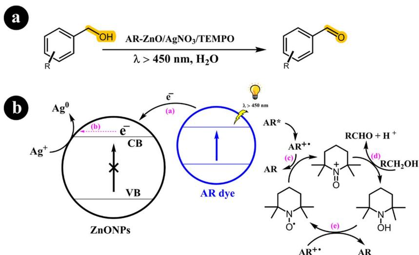
**Scheme 3** The illustration of (a) reaction conditions for the conversion of alcohols to their corresponding carbonyl compounds and (b) the catalyst design and working mechanism. Reproduced from ref. 37 with permission, copyright 2012, Royal Society of Chemistry.
