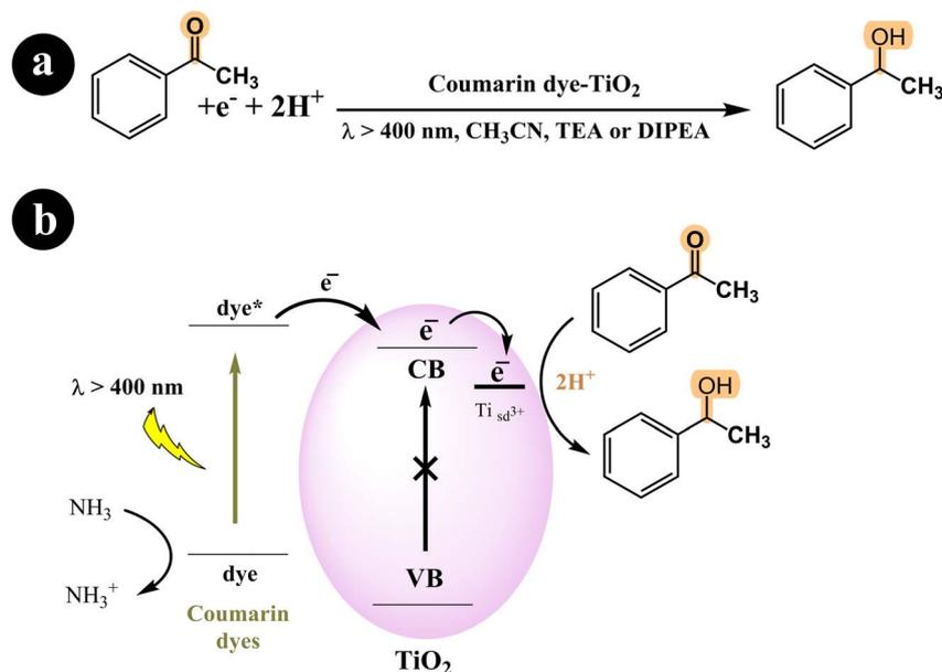
Scheme 23 (a) The reaction conditions employed for the hydrogenation of acetophenone. (b) The mechanistic pathway of photocatalysis under visible light irradiation using coumarin dyes-TiO<sub>2</sub>.
