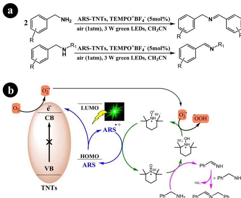
**Scheme 11** (a) reaction conditions for the aerobic oxidation of primary and secondary amines, and (b) mechanistic study for the co-catalyst utilized under green light irradiation. Reproduced with permission from ref. 49, copyright 2021, Elsevier.
