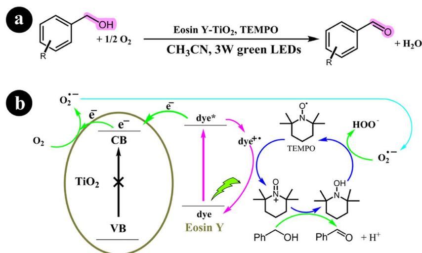
**Scheme 20** (a) Reaction conditions and (b) photocatalytic aerobic oxidation of alcohols for the eosin Y-sensitized TiO<sub>2</sub> nanoparticles. Reproduced from ref. 61, with permission, copyright 2017, Royal Society of Chemistry.
