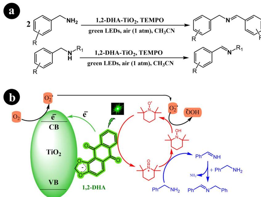
**Scheme 26** (a) 1,2-DHA-TiO<sub>2</sub>/TEMPO co-catalyst for the green light-induced photocatalytic selective oxidation of primary and secondary amines into imines using aerobic O<sub>2</sub> as the oxidizing agent, and (b) the proposed mechanism for the reactions. Reproduced with permission from ref. 76, copyright 2021, Elsevier.
