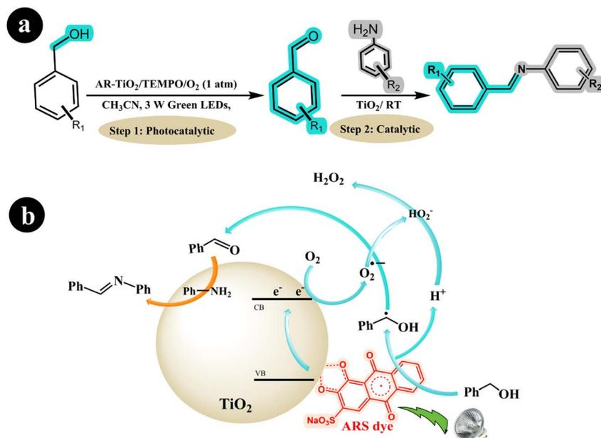
**Scheme 10** (a) The reaction conditions and (b) the proposed mechanism for synthesizing imines from amines and alcohols with air using dye-sensitized  $TiO_2$  photocatalysis under green light irradiation. Reproduced with permission from ref. 48, copyright 2019, Elsevier.
