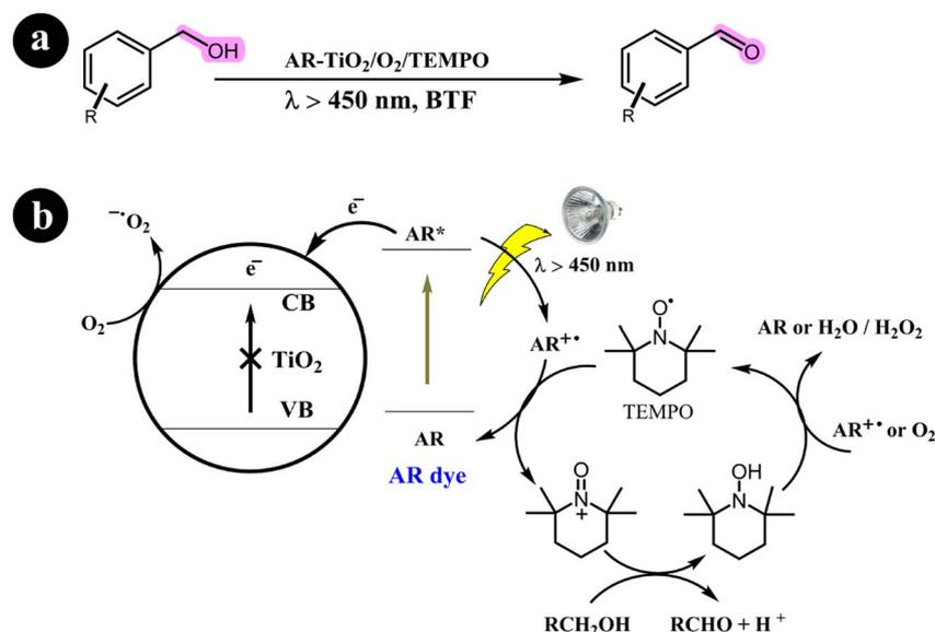
**Scheme 2** The illustration of (a) the conversion of alcohols to their corresponding aldehydes and ketones and (b) the catalyst design and working mechanism. Reproduced with permission from ref. 36. Copyright 2008, John Wiley and Sons.
