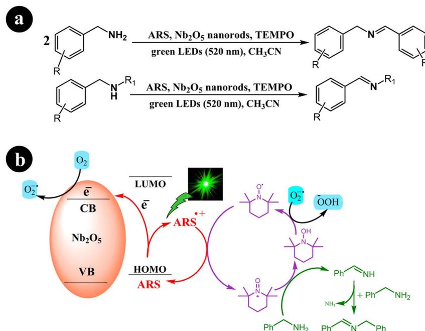
Scheme 12 (a) Reaction conditions for the aerobic oxidation of amines and (b) proposed mechanism for ARS- $\text{Nb}_2\text{O}_5$ /TEMPO co-catalysis under green LEDs irradiation. Reproduced with permission from ref. 50, copyright 2021, Elsevier.
