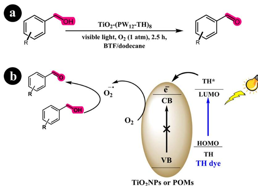
Scheme 21 (a) Reaction conditions for the aerobic oxidation of aryl alcohols to aldehydes by  $\text{TiO}_2\text{-(PW}_{12}\text{-TH)}_8$  under Blue light irradiation; (b) mechanistic pathway. Reproduced with permission from ref. 64, copyright 2017, Elsevier.
