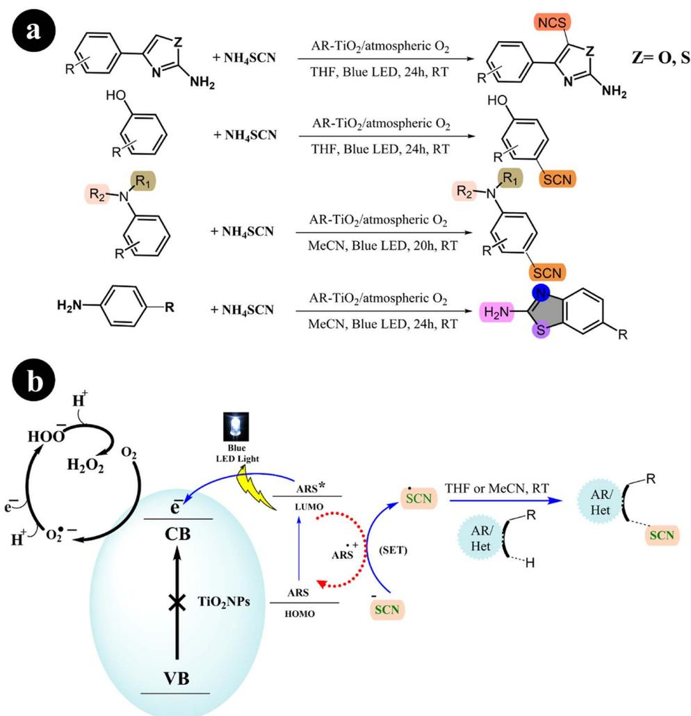
**Scheme 13** (a) Reaction conditions and (b) catalytic activation of sp<sup>2</sup> C–H bonds through thiocyanation and cyclization reactions facilitated by ARS-TiO<sub>2</sub> under blue LED irradiation. Reproduced from ref. 25, with permission, copyright 2020, Royal Society of Chemistry.
