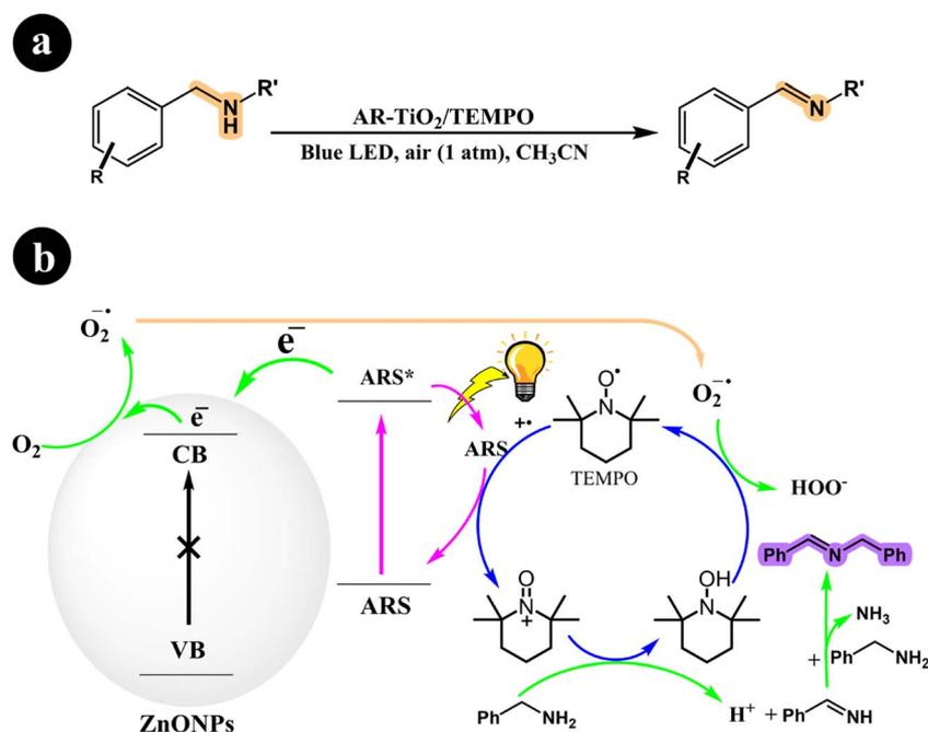
**Scheme 9** (a) Reaction conditions for the aerobic oxidation of amines to imines by ARS-TiO<sub>2</sub> using O<sub>2</sub> with TEMPO under blue light irradiation and (b) mechanistic pathway. Reproduced with permission from ref. 47, copyright 2018, Elsevier.
