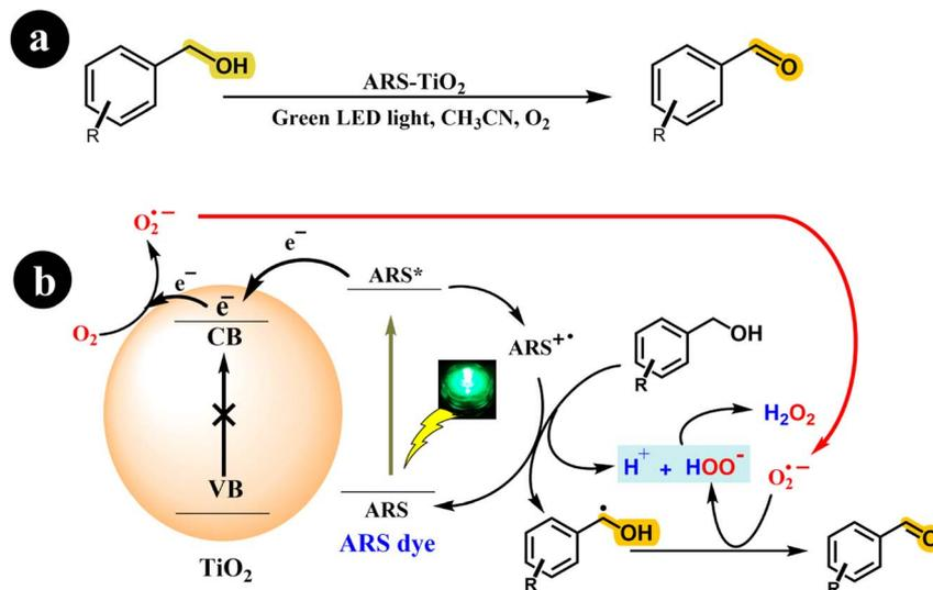
**Scheme 4** (a) The reaction conditions and (b) the proposed mechanism for the selective oxidation of benzyl alcohol with air using dye-sensitized TiO<sub>2</sub> photocatalysis under visible light irradiation. Reproduced with permission from ref. 38, copyright 2018, Elsevier.
