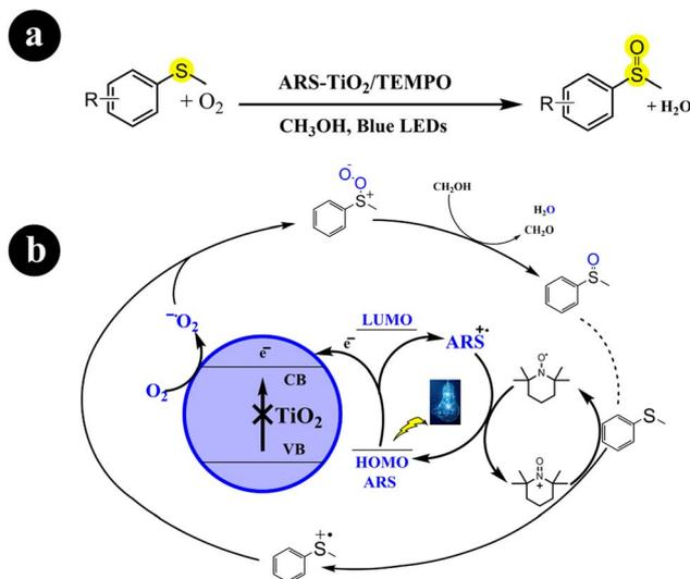
**Scheme 6** (a) Reaction conditions and (b) possible mechanism for the oxidation of sulfides to sulfoxides by ARS-TiO<sub>2</sub> under blue LED irradiation. Reproduced with permission from ref. 41. Copyright 2018, John Wiley and Sons.
