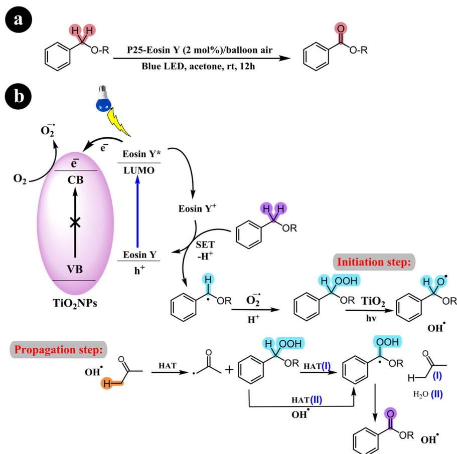
**Scheme 19** (a) Catalytic system, reaction conditions and (b) a conceivable mechanism for the aerobic oxidation process of benzyl ethers. Reproduced with permission from ref. 60. Copyright 2017, American Chemical Society.
