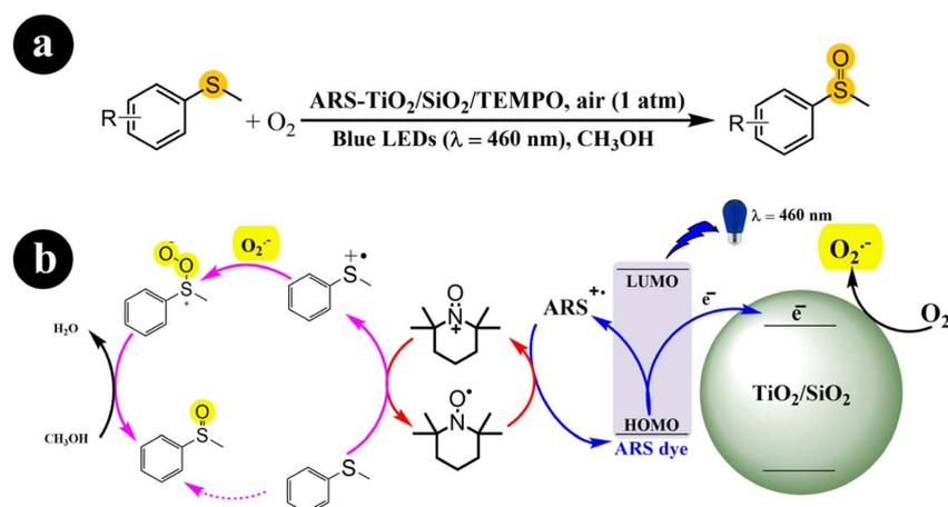
Scheme 7 (a) Reaction conditions for the aerobic oxidation of sulfides and (b) the proposed mechanism for ARS-TiO<sub>2</sub>/SiO<sub>2</sub>/TEMPO co-catalysis under blue LEDs irradiation. Reproduced with permission from ref. 43, copyright 2021, Elsevier.
