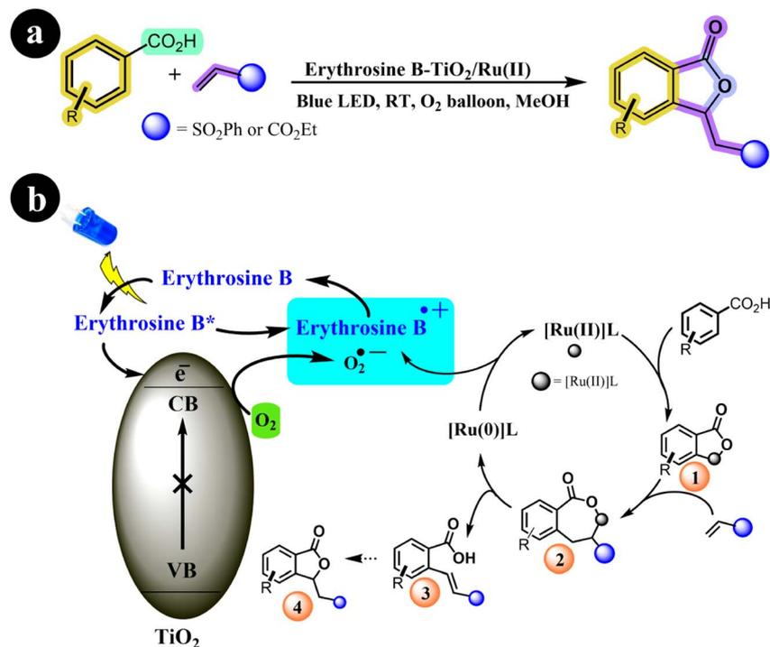
Scheme 25 (a) Reaction conditions and (b) catalytic activation of C–H bonds facilitated by Ru(II) and photoredox using O<sub>2</sub> as an oxidant under blue LED irradiation. Reproduced with permission from ref. 75. Copyright 2020, John Wiley and Sons.
