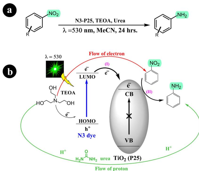
**Scheme 15** (a) The conversion reaction and the conditions for the catalysis system; (b) the reduction of nitrobenzene through photocatalysis using dye-sensitized TiO<sub>2</sub> is achieved in the presence of urea, which acts as a mediator for proton transfer. Reproduced from ref. 56 with permission, copyright 2011, Royal Society of Chemistry.
