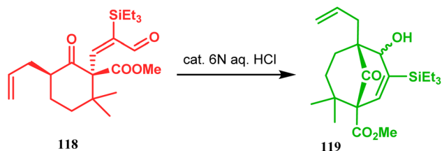
Scheme 20 Synthesis of the bicyclic core of PPAPs via the acid-catalyzed intramolecular aldolization of \alpha -silyl enal.
