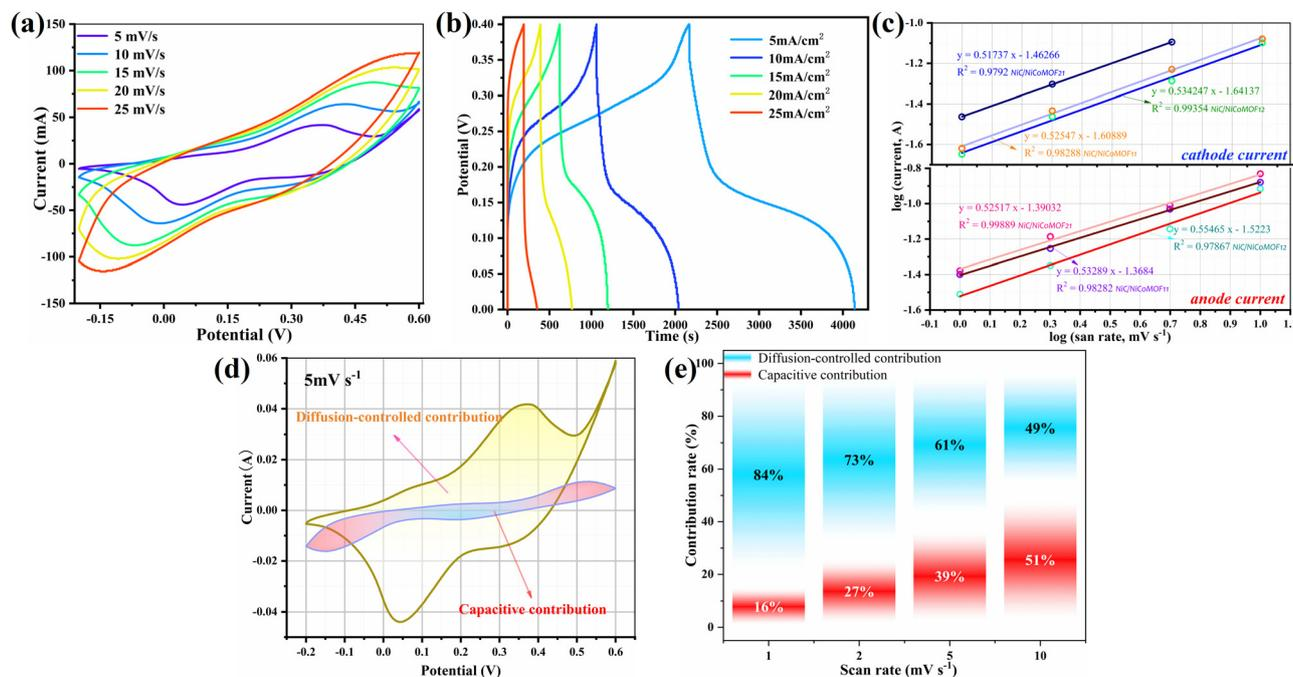
Fig. 6 CV curves of NiC/NiCoMOF21 at 5–25  $\text{mV s}^{-1}$ . (b) GCD curves of NiC/NiCoMOF21 at 5–25  $\text{mA cm}^{-2}$ . (c) Linear plot between  $\log(i)$  and  $\log(v)$  at different potentials. (d) The capacitive and diffusion-controlled contributions in the electrode process.
