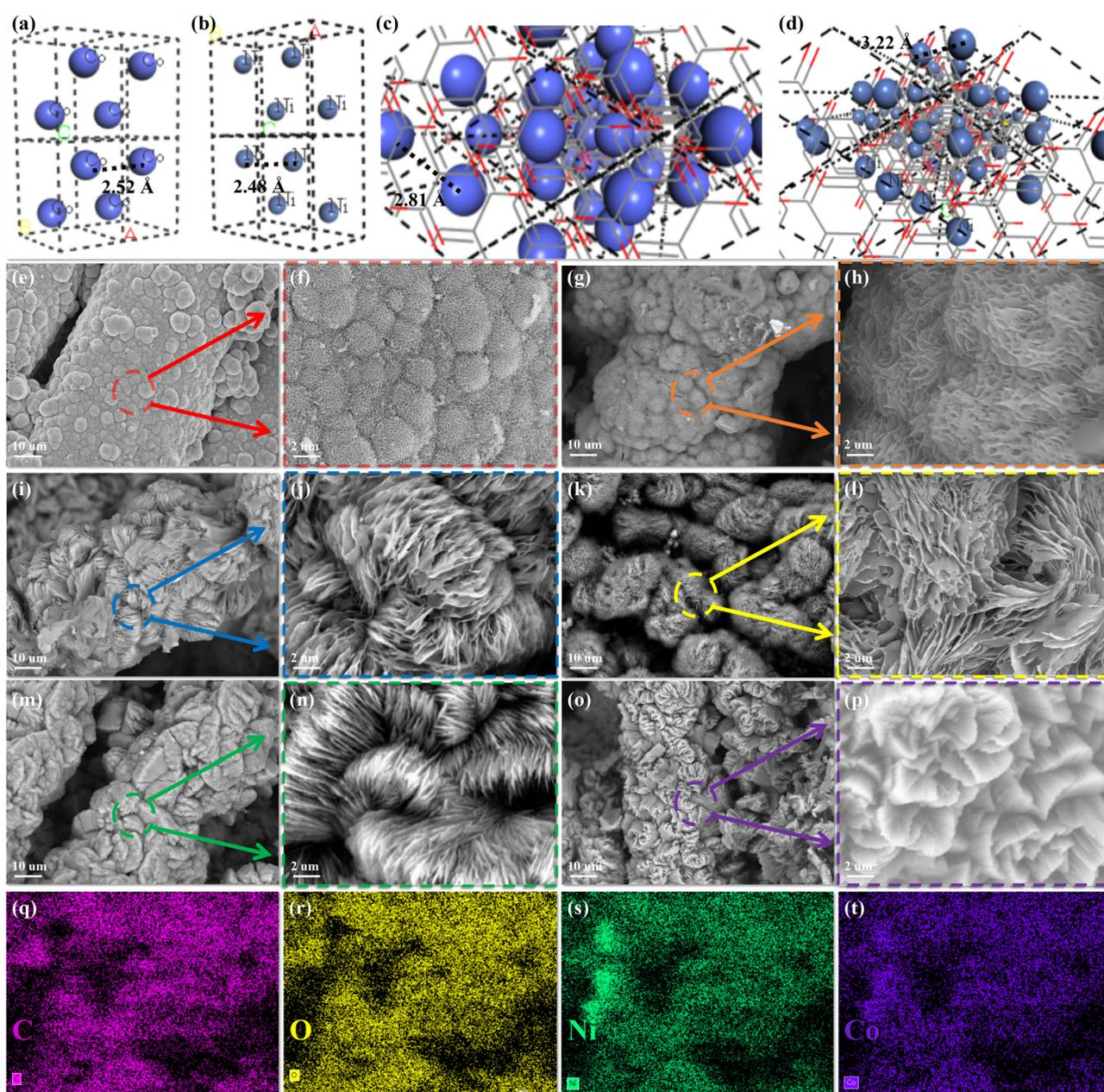
Fig. 4 (a–d) Molecular models of  $\text{Co}$ ,  $\text{Ni}$ ,  $\text{Co}-\text{MOF}$  and  $\text{Ni}-\text{MOF}$ ; (e and f) SEM images of  $\text{NiC}$ ; (g and h)  $\text{NiC}/\text{NiCoMOF10}$ ; (i and j)  $\text{NiC}/\text{NiCoMOF11}$ ; (k and l)  $\text{NiC}/\text{NiCoMOF21}$ ; (m, n)  $\text{NiC}/\text{NiCoMOF21}$ ; (o and p)  $\text{NiC}/\text{NiCoMOF01}$ . (q–t) Elemental mapping of  $\text{NiC}/\text{NiCoMOF21}$ .
