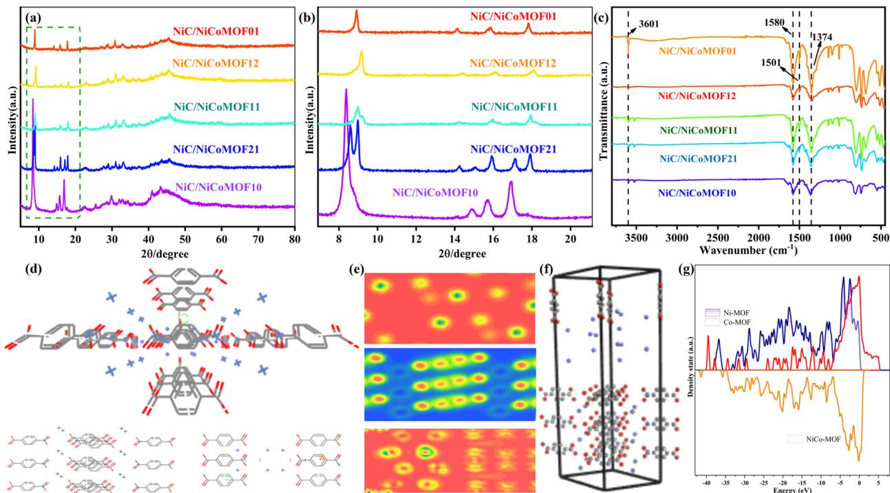
Fig. 2 (a) XRD patterns of NiCo-MOFs; (b) 5–25 degree of  $2\theta$ ; (c) FT-IR images; (d) molecular model of the NiCo-MOF composite, Ni-MOF and Co-MOF; (e and g) electron density difference maps and total density of states; (f) binding model of Ni-MOF and Co-MOF.
