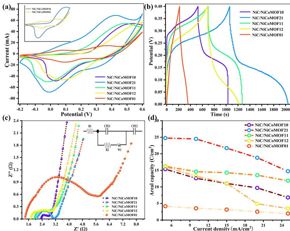
Fig. 5 (a) CV curves of the NiC/NiCo-MOFs at 5 mV s<sup>-1</sup>, the inset is NiC/NiCoMOF10 and NiC/NiCoMOF01; (b) GCD curves at 10 mA cm<sup>-2</sup>. (c) EIS plots (0.01 Hz to 100 kHz of the frequency range) and (d) areal capacities.
