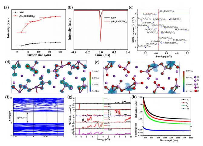
Fig. 2 (a) Phase-matching curves of  $\beta$ -Li<sub>2</sub>RbBi(PO<sub>4</sub>)<sub>2</sub>. (b) SHG intensity of  $\beta$ -Li<sub>2</sub>RbBi(PO<sub>4</sub>)<sub>2</sub> and KDP. (c) SHG response of all Bi-based phosphates. (d and e) Veocc (d) and veunocc (e) states of the largest SHG tensor  $d_{22}$ . (f) Electronic structure of  $\beta$ -Li<sub>2</sub>RbBi(PO<sub>4</sub>)<sub>2</sub>. (g) Density of states (DOS) and projected DOS (PDOS) plots. (h) Refractive indices and birefringence.
