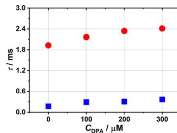
**Fig. 7** The lifetimes of **4** in  $\text{H}_2\text{O}$  and  $\text{D}_2\text{O}$  with different DPA concentrations (blue dots represent the  $\text{H}_2\text{O}$  system and red dots represent the  $\text{D}_2\text{O}$  system).
