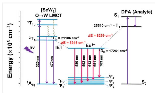
**Fig. 8** The energy level diagram exhibiting the proposed energy transfer pathways from the excited triplet states ( $T_1$ ) of  $\{SeW_9\}$  and DPA ligands to the  $^5D_0$  state of the  $Eu^{3+}$  ions. IET is internal energy transfer.
