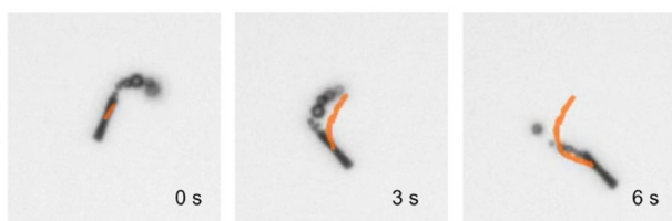
A Time lapse of \text{MnO}_2 micromotor trajectories at 2 wt. % \text{H}_2\text{O}_2
