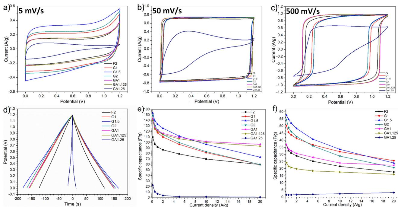
Fig. 4 Electrochemical performance of MC electrodes: (a–c) CV test at scan rates of 5, 50, and 500  $\text{mV s}^{-1}$ , (d) galvanostatic charge/discharge at  $0.5 \text{ A g}^{-1}$ , (e) gravimetric capacitance in 6 M KOH electrolyte; (f) gravimetric capacitance in  $[N_{2220}][INTf_2]/ACN$  electrolyte.
