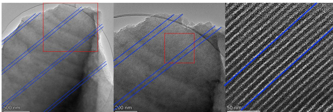
**Fig. 5** TEM images of ordered mesopore channels in glyoxal-derived sample G1.5 (double blue lines indicate the orientation of 5 neighbouring mesopore channels, which reached a magnitude of micrometres in depth).
