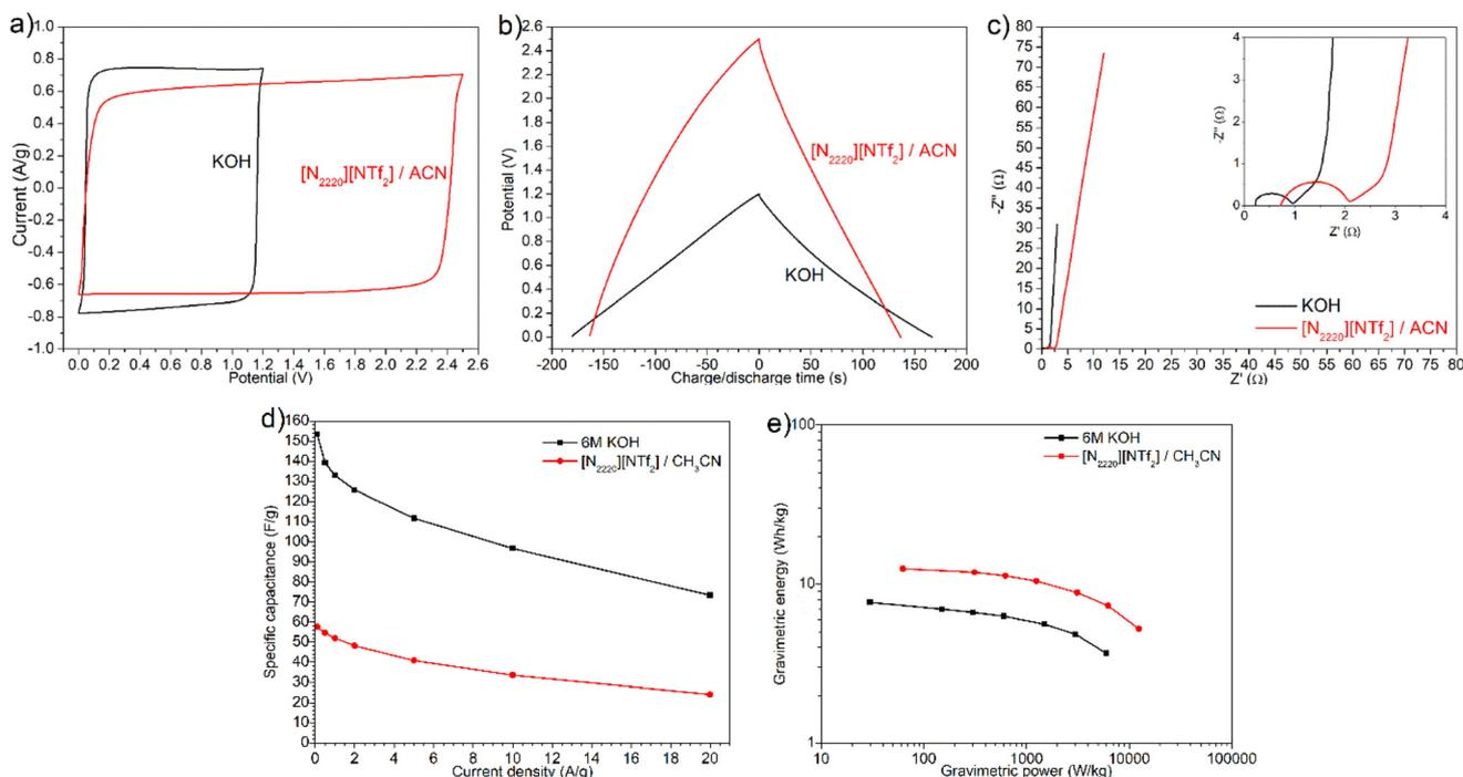
**Fig. 6** G1.5 electrode in two different electrolytes: (a) CV test at  $50 \text{ mV s}^{-1}$ , (b) galvanostatic charge/discharge at  $0.5 \text{ A g}^{-1}$ , (c) Nyquist plot, (d) gravimetric specific capacitance, and (e) energy density, respectively.
