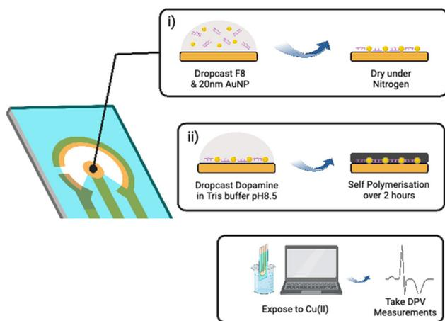
**Fig. 3** DNAzyme based electrochemical biosensor for  $\text{Cu}(\text{II})$  is prepared by drop casting DNAzyme/substrate complex and rate enhancing Au NPs to the surface of electrode (i) followed by addition of dopamine and self-polymerisation resulting in PDA coating. (ii) Sensor is prepared within 2 hours after which  $\text{Cu}(\text{II})$  detection can be performed using differential pulse voltammetry (DPV).
