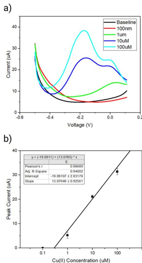
**Fig. 6** (a) DPV response curves for polydopamine entrapped F8 sensor in increasing concentrations of copper from 0 to  $100 \mu\text{M}$ . All measurements were taken in PBS after 15 min with stirring ( $100 \text{ rpm}$ ). (b) Peak current measured in sensing range of  $-0.4$  V to  $0.1$  V for different copper concentrations with a linear fit after subtracting a baseline taken in PBS only.
