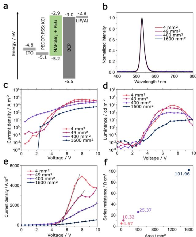
**Fig. 2** (a) Device architecture and energy levels as used previously in ref. 14, (b) electroluminescence spectra, (c) current densities, (d) luminance–voltage characteristics for all devices, (e) extraction of series resistance and (f) active area dependent series resistance.
