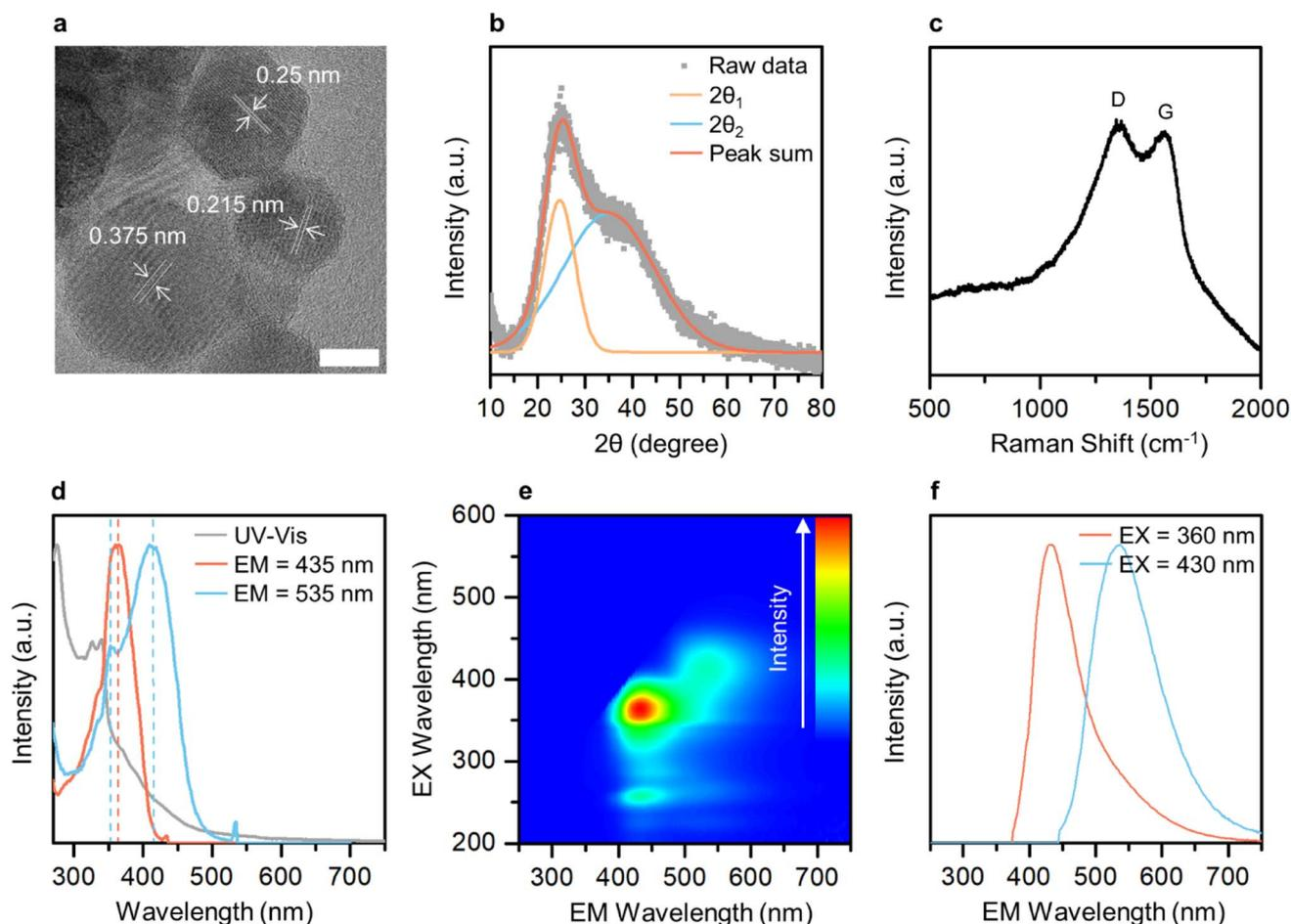
**Fig. 2** (a) High-resolution TEM image of GE-CDs. (scale bar, 10 nm). (b) XRD pattern of GE-CDs. (c) Raman spectrum of GE-CDs. (d) Normalized UV-visible absorption and PL excitation spectra of GE-CDs. (e) PL emission contour map of GE-CDs. (f) PL emission spectra of GE-CDs at excitation wavelengths of 360 and 430 nm. "EX" and "EM" designate excitation and emission, respectively.
