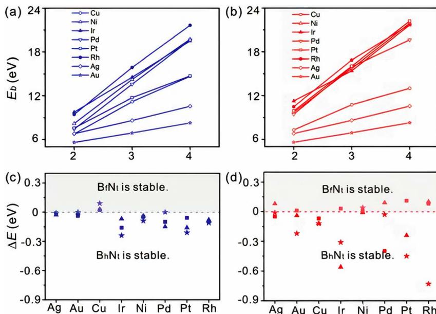
Fig. 3 Binding energies as a function of BN clusters terminated with (a) N and (b) B atoms. The difference in formation energy between  $B_hN_t$  and  $B_fN_t$  of (c) N and (d) B terminated BN clusters. Squares, stars, and triangles represent the cluster size of 2, 3, and 4, respectively.<sup>180</sup>
