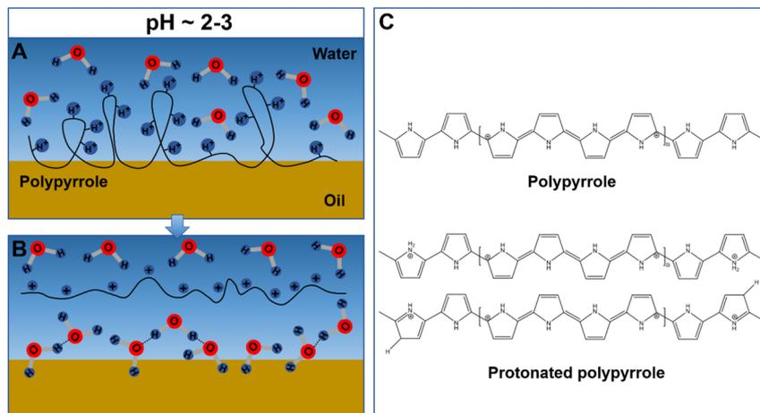
**Scheme 3** pH-dependent adsorption and desorption of polypyrrole at the oil–water interface. Polypyrrole is firstly protonated by the protons ( $H^+$ ) at pH  $\sim 2-3$  (A), and subsequently adopts an extended conformation as a result of the electrostatic interaction, and desorbs from the oil–water interface due to a reduction in free energy (B). (C) The chemical structures of the pristine polypyrrole and protonated polypyrrole.
