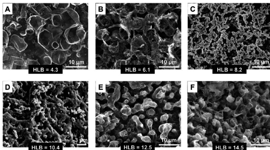
**Fig. 1** Changes in the morphology of polypyrrole synthesized by interfacial polymerization with the addition of mixture surfactants with different HLB values. The morphologies of the as-synthesized polypyrrole alter from ruptured vesicle-like (A and B) to network-like (C and D), and eventually to coral-like (E and F) as the HLB value of the surfactant increased. Reproduced from ref. 34, with permission from Elsevier, 2018.
