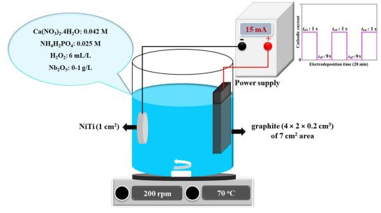
Schematic illustration of the electrolyte composition and electrodeposition parameters in the present work
