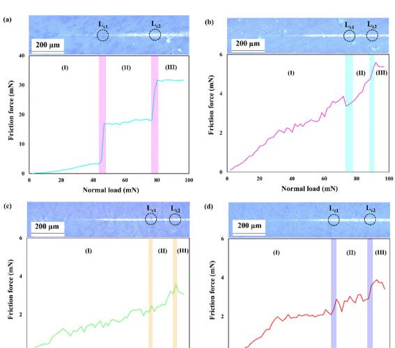
Fig. 10 Obtained curves from nanoscratch testing along with the corresponding panorama images of track traces (at the magnification of  $100 \times$ ): (a) S1, (b) S2, (c) S3, and (d) S4.
