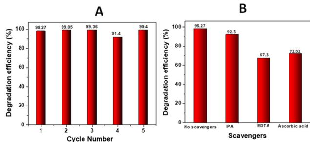
Fig. 10 (A) Degradation efficiency after 5 cycles of TC-HC degradation in the presence of ZNTC\_600. (B) Degradation efficiency of TC-HC in the presence of ZNTC\_600 with different scavengers.
