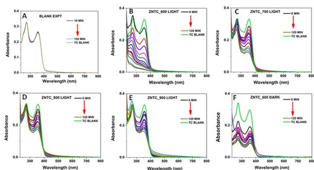
Fig. 4 UV-Vis absorbance variations of TC-HC for 120 minutes in (A) the absence of catalyst and the presence of light and (B) ZNTC\_600. (C) ZNTC\_700, (D) ZNTC\_800 and (E) ZNTC\_900, and (F) in the dark in the presence of ZNTC\_600.
