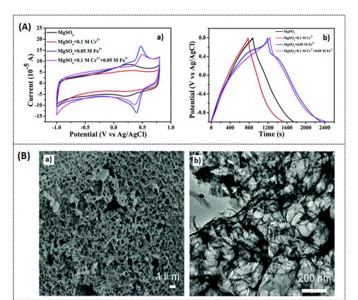
Fig. 15 (A) (a and b) CV response of optimal composite BPGC at different electrolyte medium at a scan rate 5 mV s<sup>-1</sup>, GCD response at 0.5 A g<sup>-1</sup> current density. (B) (a and b) SEM and TEM images of BPGC. Reproduced with permission, 96 Copyright (2022), Royal Society of Chemistry
