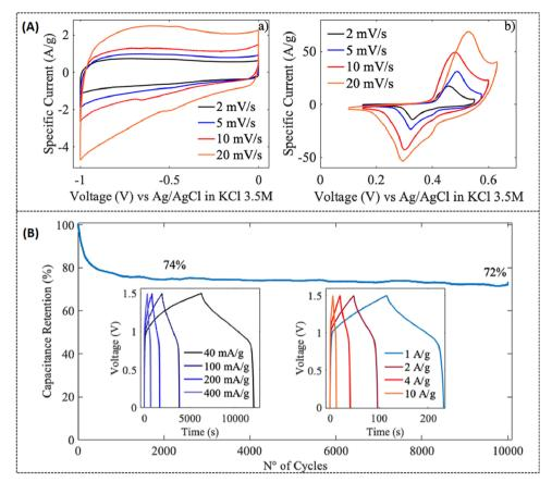
Fig. 16 (A) (a and b) CV response of TEGO and Ni-TEGO at different scan rates, (B) capacitance retention response of ASCs over 10 000 cycles at 1 A g<sup>-1</sup> current density inset: with GCD curves at different applied current density. Reprinted with permission, <sup>97</sup> Copyright (2022) from Elsevier.
