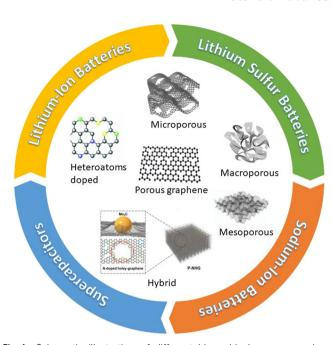
Fig. 1 Schematic illustration of different hierarchical porous graphene utilized for lithium-ion batteries, lithium-sulfur batteries, sodium-ion batteries, and supercapacitors. Porous structures are reprinted with permission from ref. 21 (micropore),<sup>22</sup> (macropore),<sup>23</sup> (mesopore),<sup>24</sup> (hybrid),<sup>25</sup> (heteroatoms doped).
