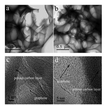
Fig. 14 TEM images of (a and c) nitrogen doped porous carbon (b and d), porous GO/PANI nanorods array/GO electrode (GPGC) composite. Reprinted with permission, 95 Copyright (2021) from Elsevier.
