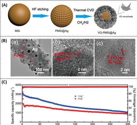
Fig. 5 (A) Schematic representation of the as-prepared VG-PMS@Ag, (B) (a-c) TEM images of the PMS@Ag composite, interplanar spacing of Ag in PMS@Ag, interplanar spacing of Silicon in PMS@Ag. (C) Long-term cycling activity of the VG-PMS@Ag electrode at different applied current densities. Reprinted with permission, 42 Copyright [2022] American Chemical Society.
