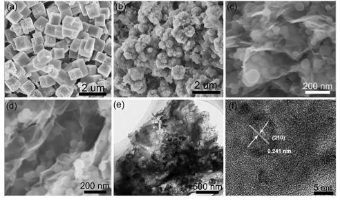
Fig. 11 SEM morphology of (a) PB, (b) FeS2-C, (c) PB/r-GO, (d) FeS2-C/RG, (e and f) TEM and HRTEM images of optimal FeS2-C/RG. Reprinted with permission,<sup>73</sup> Copyright (2020) from Elsevier.
