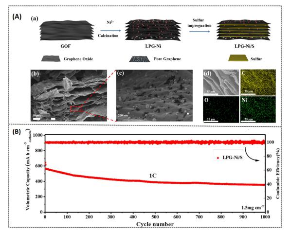
Fig. 8 (A) (a) Schematic representation of the as-prepared LPG-Ni/S composite, (b-d) cross-sectional FESEM images of LPG-Ni at various magnifications and its corresponding elemental mapping of C, O, Ni. (B) Long-term cycling performance of the LPG-Ni/S cathode material. Reprinted with permission, <sup>63</sup> Copyright (2022) from Elsevier.
