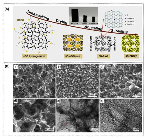
Fig. 6 (A) Schematic illustration of the preparation process of 3D-PNG/S composites, (B) (a and b) SEM images of 3D-rGO, 3D-rGO@ures, (c and d) lowhigh-magnification of 3D-PNG (e and f) TEM image of 3D-PNG, HRTEM image of the marked area in. Reprinted with permission, <sup>56</sup> Copyright (2019) from Flsevier
