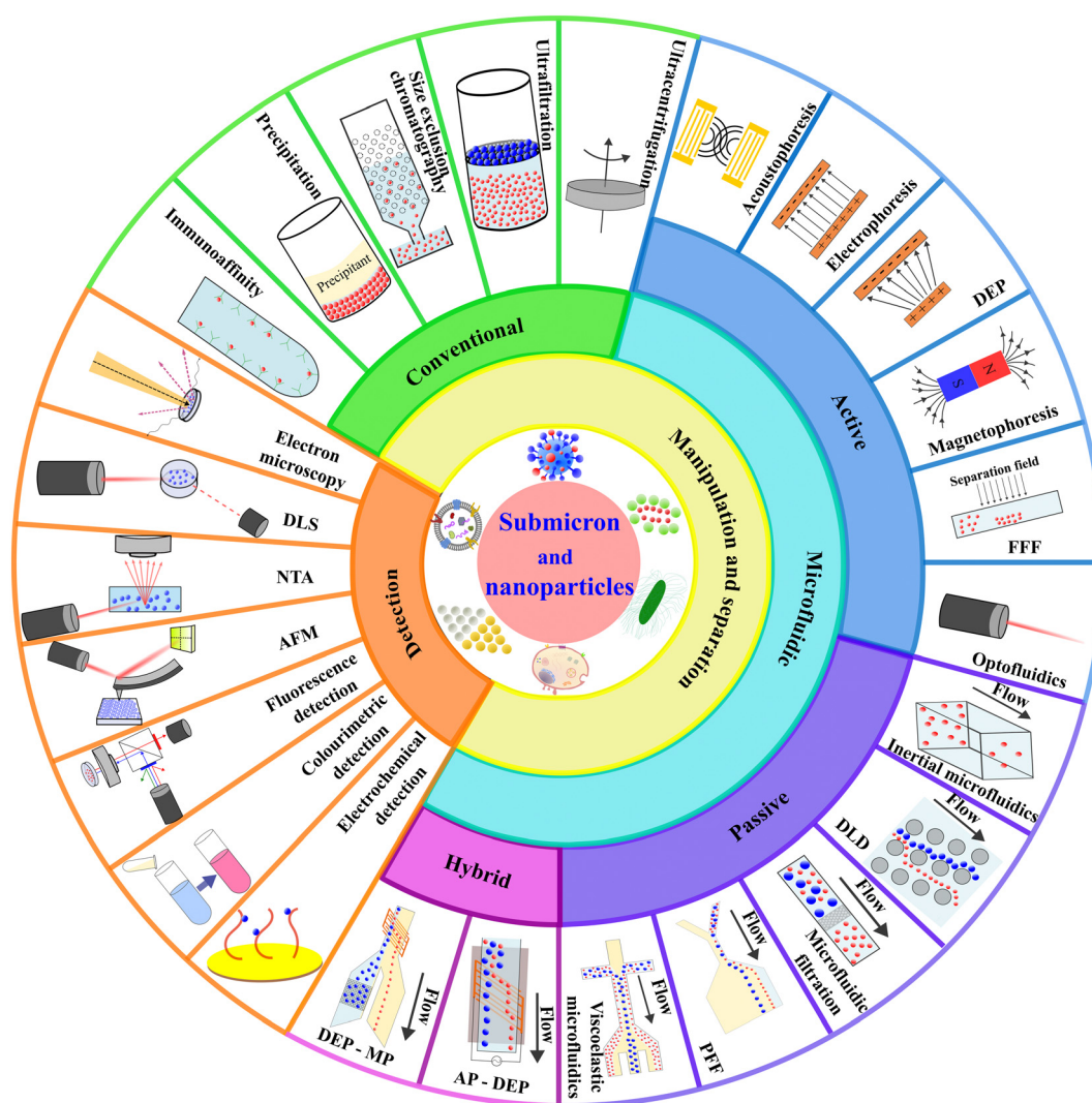
Fig. 1 An overview of submicron and nanoparticle manipulation, separation and detection techniques. Manipulation and separation can be mainly categorised as conventional and microfluidic technologies. Microfluidic technologies can be further subdivided into active, passive and hybrid techniques according to the manipulating forces. Abbreviations are DEP (dielectrophoresis), FFF (field flow fractionation), DLD (deterministic lateral displacement), PFF (pinched flow fractionation), AP-DEP (acoustic-dielectrophoresis), DEP-MP (dielectrophoresis-magnetophoresis), AFM (atomic force microscopy), NTA (nanoparticle tracking analysis), and DLS (dynamic light scattering).
