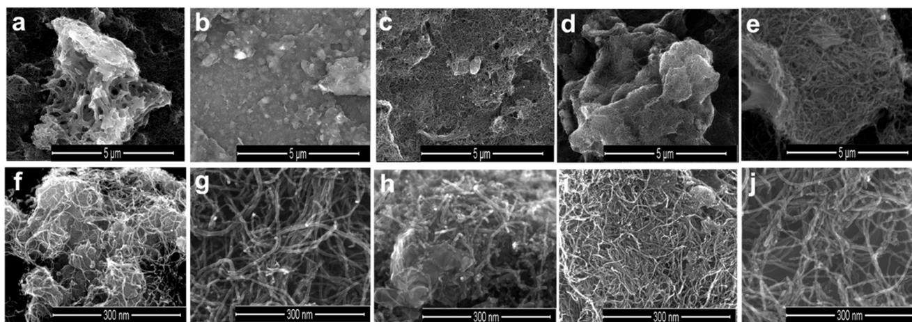
**Fig. 2** SEM images captured for (a and f) ZNT-900, (b and g) Fe-ZNT-900, (c and h) Co-ZNT-900, (d and i)  $\text{Fe}_1\text{Co}_1$ -ZNT-900 and (e and j)  $\text{Fe}_1\text{Co}_2$ -ZNT-900 catalysts at different resolutions.
