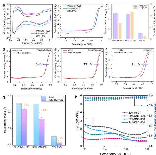
**Fig. 4** (a) Cyclic voltammograms; (b) polarization curves and (c) mass activity (MA) and specific activity (SA) for PtNi/CNF-1200, PtNi/KBC-600 and 20% Pt/C; polarization curves for (d) PtNi/CNF-1200; (e) PtNi/KBC-600 and (f) 20% Pt/C before and after 5000 cycles in a high potential range of 1.0–1.5 V; (g) MA comparison of PtNi/CNF-1200, PtNi/KBC-600, and 20% Pt/C before and after 5000 potential cycles; (h) H<sub>2</sub>O<sub>2</sub> yield and electron transfer number.
