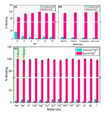
Fig. 6 Histograms of binding and performance studies of M-g-CN: (a) binding efficiencies at different pHs (pH 2-10). (b) Binding efficiencies in various aqueous matrices (marine, stream, precipitation, and ultrapure). (c) Binding efficiency determination of Hg<sup>2+</sup> towards M-g-CN in the presence of interfering ions.
