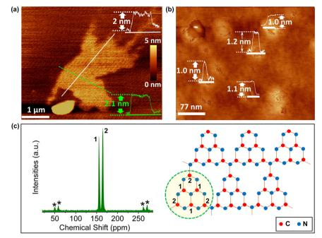
Fig. 2 (a) AFM image of q-CN nanosheet with sectional profile measurement showing height and thickness profiles (nm). (b) AFM images of nanosheets with respective height profiles at different locations. (c) Solid-state <sup>13</sup>C NMR spectra of as-prepared g-CN and its idealized structure showing heptazine tectonic units
