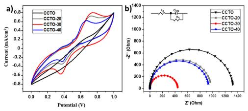
Fig. 6 (a) Cyclic voltammetry curves obtained using CCTO, CCTO-20, CCTO-30 and CCTO-40 as electrodes in 1 M KOH (scan rate = 25 mV s $^{-1}$ ). (b) Nyquist plots showing the electrochemical impedance spectroscopy data for CCTO, CCTO-20, CCTO-30 and CCTO-40.
