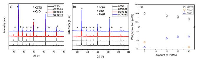
Fig. 3 (a) XRD patterns of CCTO pellets prepared using different amounts of PMMA (0, 20, 30, and 40 wt%). (b) XRD patterns of the same samples after powdering. (c) Weight fraction of the formed crystalline phases (Rietveld analysis of the XRD data for the powdered samples).
