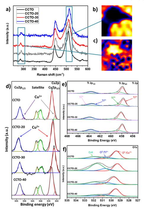
Fig. 4 (a) Raman shifts of the CCTO samples prepared using different PMMA amounts (0, 20, 30, and 40 wt%). (b and c) Raman maps: (b) 510 cm $^{-1}$  (CCTO) and (c) 291 cm $^{-1}$  (CuO). (d-f) High-resolution XPS spectra of (d) Cu  $2p_{3/2}$ , (e) Ti  $2p_{3/2}$ , and 9f) O 1s for the CCTO samples prepared using different PMMA amounts (0, 20, 30, and 40 wt%).
