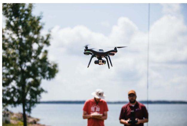
Fig. 2 A close-up image of the multirotor sUAS that was used to measure wind velocity at onshore and offshore locations in Grant Lake St. Marys, Ohio on August 5th and 6th, 2019.
