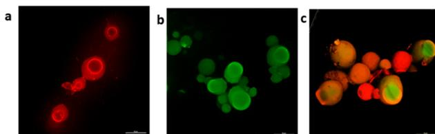
**Fig. 2** Confocal microscopy of glyoxyl-agarose particles immobilizing a: rhodamine-labelled RN (5 mg  $g_{\text{resin}}^{-1}$ ); b: fluorescein-labelled HOR (1 mg  $g_{\text{resin}}^{-1}$ ); c: rhodamine-labelled RN and fluorescein-labelled HOR (5 mg<sub>RN</sub>  $g_{\text{resin}}^{-1}$ , 1 mg<sub>HOR</sub>  $g_{\text{resin}}^{-1}$ ). Magnification 20 $\times$ .
