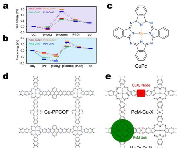
**Fig. 9** Free energy diagrams for CO production on metallophthalocyanine-based Cu MOFs considering the a) concerted PCET mechanism and b) sequential PCET mechanism. Free energies are relative to desorbed CO<sub>2</sub>. Adapted with permission from Meng *et al.*<sup>118</sup> Copyright 2020 American Chemical Society. The structures of c) molecular PcCu, d) Cu-PPCOF, and e) PcM-Cu-X.
