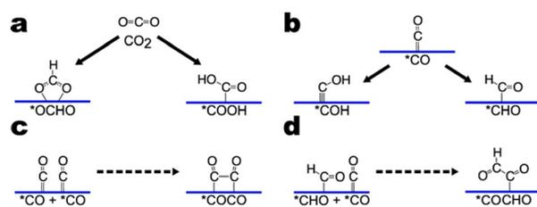
**Fig. 2** Selected sub-pathways of CO<sub>2</sub>RR. a) Proton-coupled electron transfer of CO<sub>2</sub> to \*OCHO or \*COOH. b) Proton-coupled electron transfer of \*CO to \*COH or \*CHO. c) \*CO dimerization reaction. d) C-C coupling of \*CHO and \*CO. Solid lines denote proton-coupled electron transfers. Dashed arrows denote coupling reactions.
