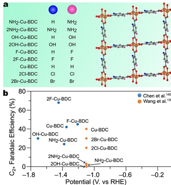
Fig. 18 a) Depiction of the general structure of the series of substituted 1,4-benzene dicarboxylate-based MOFs studied by Chen *et al.*<sup>140</sup> and Wang *et al.*<sup>139</sup> Grey, orange, red, and white spheres denote carbon, copper, oxygen, and hydrogen atoms. Pink and blue spheres denote variable functional groups. b) Faradaic efficiencies for C<sub>2+</sub> products by X-Cu-BDC MOFs studied by Chen *et al.*<sup>140</sup> and Wang *et al.*<sup>139</sup>
