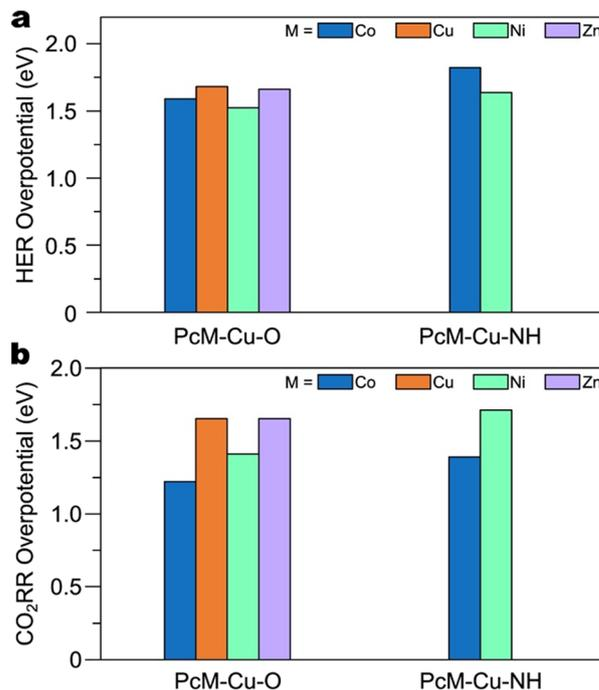
**Fig. 12** DFT-calculated overpotentials for a) CO and b)  $\text{H}_2$  production on the SBUs of various PcM–Cu–X MOFs. Data for Co- and Ni-bearing MOFs from Meng *et al.*<sup>118</sup> Data for PcCu–Cu–O and PcZn–Cu–O from Zhong *et al.*<sup>121</sup>
