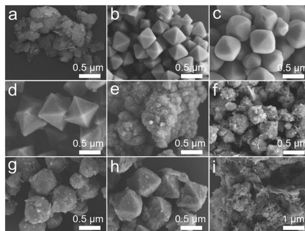
**Fig. 3** SEM images of  $\text{ZnIn}_2\text{S}_4$  (a) UiO-66- $\text{NH}_2$  (b), UiO-66-OH (c), UiO-66 (d), UiO-66- $(\text{OH})_2$  (e), Z-UN (f), Z-UOH (g), Z-U (h) and Z-U( $\text{OH})_2$  (i).
