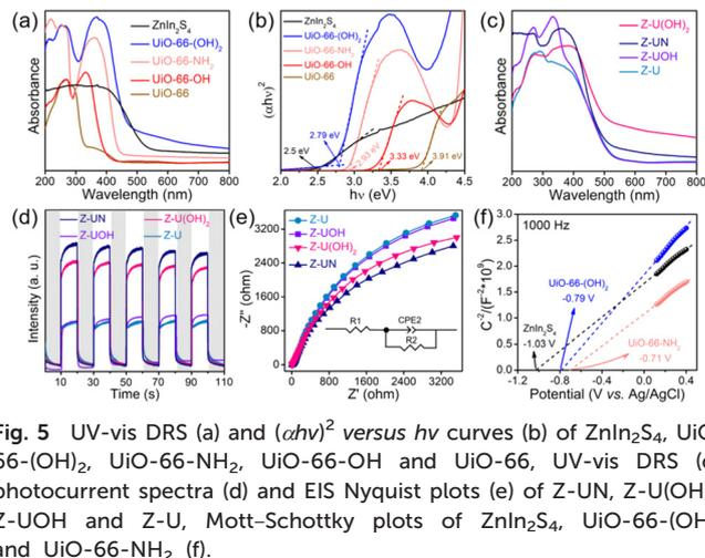
**Fig. 5** UV-vis DRS (a) and  $(\alpha hv)^2$  versus  $h\nu$  curves (b) of ZnIn<sub>2</sub>S<sub>4</sub>, UiO-66-(OH)<sub>2</sub>, UiO-66-NH<sub>2</sub>, UiO-66-OH and UiO-66, UV-vis DRS (c), photocurrent spectra (d) and EIS Nyquist plots (e) of Z-UN, Z-U(OH)<sub>2</sub>, Z-UOH and Z-U, Mott-Schottky plots of ZnIn<sub>2</sub>S<sub>4</sub>, UiO-66-(OH)<sub>2</sub> and UiO-66-NH<sub>2</sub> (f).
