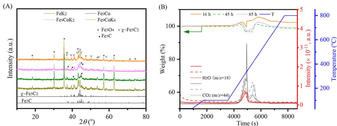
Fig. 3 (A) XRD patterns of the spent catalysts with 16 h TOS and (B) TGA-MS profiles of the spent  $\text{Fe}_9\text{CoK}_6$  catalysts with different TOS at 300 °C with a  $\text{H}_2$  to  $\text{CO}_2$  ratio of 2 and GHSVs of (A) 3600  $\text{mL g}_{\text{cat}}^{-1} \text{h}^{-1}$  and (B) 7200  $\text{mL g}_{\text{cat}}^{-1} \text{h}^{-1}$ .
