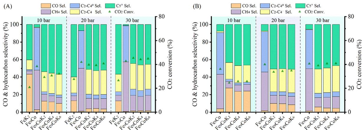
Fig. 5 Catalytic performance of  $\text{Fe}_9\text{CoK}$  catalysts with different K loadings under different pressures at 300 °C with a  $\text{H}_2$  to  $\text{CO}_2$  ratio of 2 and GHSVs of (A) 3600  $\text{mL g}_{\text{cat.}}^{-1} \text{h}^{-1}$  and (B) 7200  $\text{mL g}_{\text{cat.}}^{-1} \text{h}^{-1}$ .
