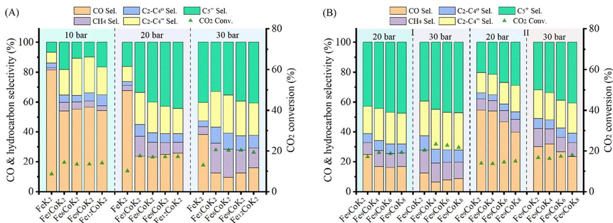
Fig. 4 Catalytic performance of Fe-Co catalysts under different pressures at 250 °C with a  $\text{H}_2$  to  $\text{CO}_2$  ratio of 2 and GHSVs of 3600  $\text{mL g}_{\text{cat}}^{-1} \text{h}^{-1}$  (A and B-zone I) and 7200  $\text{mL g}_{\text{cat}}^{-1} \text{h}^{-1}$  (B-zone II).
