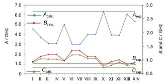
Fig. 3 The rotational constants  $A_{\text{calc.}}$ ,  $B_{\text{calc.}}$  and  $C_{\text{calc.}}$  of different conformers of ethyl butyrate calculated at the MP2/6-311++G(d,p) level of theory in comparison with those of the observed conformer which belongs to the  $C_s$  point group (horizonal lines). Lines connecting the calculated rotational constants are only for a better tracing
