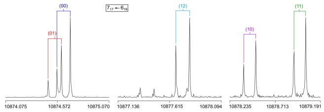
Fig. 5 High resolution measurements of the a-type transition  $7_{17} \leftarrow 6_{16}$  with its five torsional species (00), (10), (01), (11), and (12). The frequencies are in MHz. The brackets indicate Doppler pairs. The spectra were recorded at 10 874.75 MHz and 10 877.75 MHz with 50 co-added free induction decays (FIDs), and at 10 878.97 MHz with 116 co-added FIDs.
