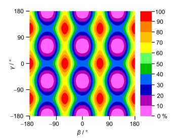
Fig. 4 Two-dimensional potential energy surface of syn-2A5MT calculated at the MP2/6-31G(d,p) level of theory in dependence of the dihedral angles  $\beta$  and  $\gamma$ , which were varied in a grid of 10° while all other geometry parameters were optimised. The colour code gives the relative energy (in percent) on a scale between the minimum  $E_{min} = -743.368307$  hartree (0%) and the maximum  $E_{\text{max}} = -743.365928$  hartree (100%)
