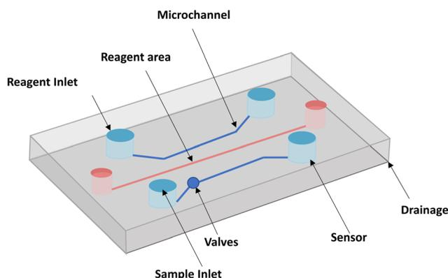
**Fig. 3** The general structure of a microfluidic chip.
