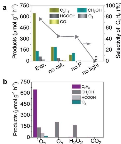
Fig. 2 Photocatalytic performance of the TiO<sub>2</sub>-<sup>1</sup>O<sub>2</sub> system under solar light irradiation: (a) comparison of this work (Exp.) and control experiments by varying conditions (no light, no P, and no cat.); (b) products obtained with different oxidants (<sup>1</sup>O<sub>2</sub>, O<sub>2</sub>, H<sub>2</sub>O<sub>2</sub>, and CO<sub>2</sub>).
