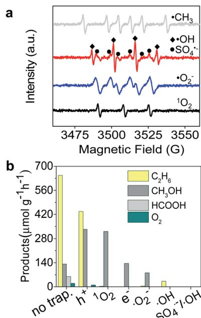
Fig. 3 (a) ESR spectra of  $\cdot\text{CH}_3$ ,  $\cdot\text{OH}$ ,  $\text{SO}_4^{\cdot-}$ , and  $\cdot\text{O}_2^-$  radicals produced after photocatalytic reaction for 10 min. (b) Products of  $\text{CH}_4$  conversion after adding scavengers *para*-quinone,  $\text{K}_2\text{Cr}_2\text{O}_7$ ,  $\text{Na}_2\text{C}_2\text{O}_4$ , and salicylic acid in the reaction system for trapping  $\cdot\text{O}_2^-$ ,  $\text{e}^-$ ,  $\text{h}^+$ , and  $\cdot\text{OH}$ , respectively.
