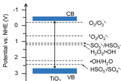
Fig. 1 Band structure of TiO<sub>2</sub> (Degussa P25) and redox potentials of reactive oxygen species.
