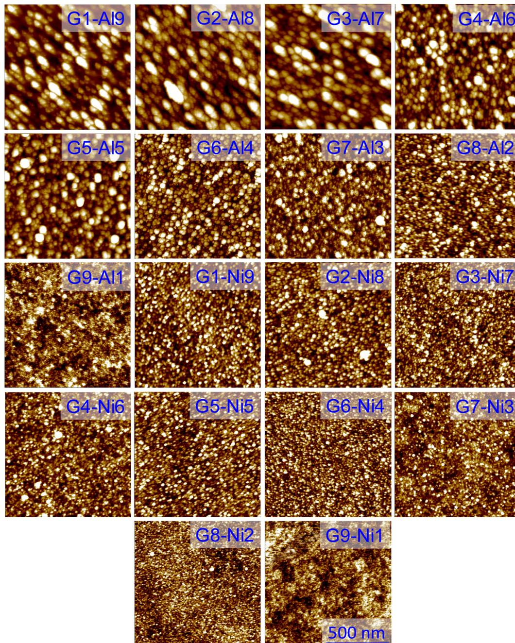
Fig. 5 Surface topography (area:  $1 \times 1 \mu\text{m}$ ) of the G:Al and G:Ni electrodes measured using AFM in noncontact mode.
