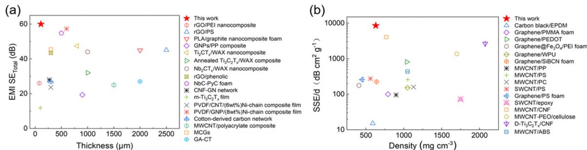
Fig. 4 Comparison of the EMI shielding performance. (a) EMI SE<sub>Total</sub> versus the thickness of Ti<sub>3</sub>C<sub>2</sub>T<sub>x</sub>/MLPAN and other EMI shielding materials from the references. (b) Thickness-normalized specific SE (SSE/d) of Ti<sub>3</sub>C<sub>2</sub>T<sub>x</sub>/MLPAN with a density of 639.0 mg cm<sup>-3</sup> and other EMI shielding materials from the references.
