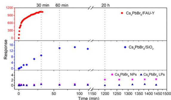
**Fig. 5** Response changes of  $\text{Cs}_4\text{PbBr}_6/\text{FAU-Y}$ ,  $\text{Cs}_4\text{PbBr}_6/\text{SiO}_2$ ,  $\text{Cs}_4\text{PbBr}_6$  NPs, and  $\text{Cs}_4\text{PbBr}_6$  LPs upon exposure to 45% RH condition.
