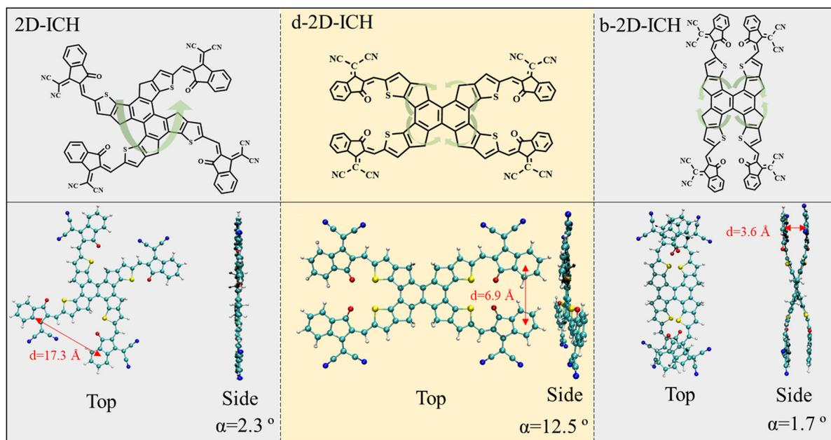
Fig. 1 Chemical structures and top/side view for the optimized structures of **2D-ICH**, **d-2D-ICH**, and **b-2D-ICH**. Dihedral angle ( $\alpha$ ) and center distance ( $d$ ) of the nearest adjacent end groups are listed at the bottom.
