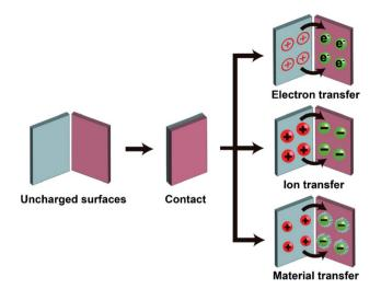
Fig. 2 Charge generation at the solid-solid interface. Scheme illustrates the three fundamental mechanisms (i.e., electron transfer, ion transfer, and material transfer) of contact electrification between two solid surfaces
