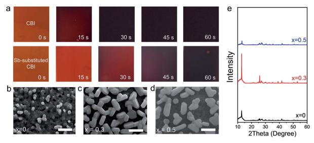
Fig. 1 (a) Photographs of CsBi<sub>3</sub>I<sub>10</sub> (CBI) and Cs(Bi<sub>0.7</sub>Sb<sub>0.3</sub>)<sub>3</sub>I<sub>10</sub> (CBSI-3) films with different thermal annealing duration. SEM images of (b) CBI, (c) CBSI-3, and (d) CBSI-5 films, the scale bar corresponds to 500 nm. (e) XRD patterns of CBI (x = 0), CBSI-3 (x = 0.3), and CBSI-5 (x = 0.5) films. (All films illustrated here are synthesized from DMF/DMSO mixed solvent with the volume ratio of 9:1).
