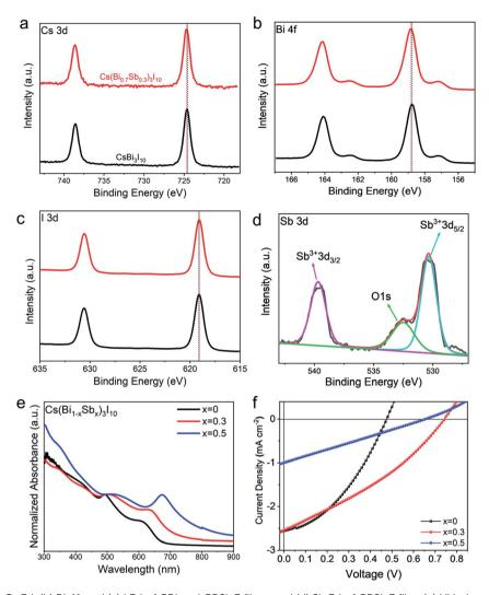
Fig. 2 XPS spectra of (a) Cs 3d, (b) Bi 4f, and (c) I 3d of CBI and CBSI-3 films, and (d) Sb 3d of CBSI-3 film, (e) UV-vis spectra of CBI, CBSI-3, and CBSI-5 films on the ITO/PEDOT substrate. (f) J-V curves of CBI, CBSI-3, and CBSI-5 devices with an inverted device architecture (ITO/PEDOT/ CSBI/PCBM/bathocuproine (BCP)/Ag) measured under illumination (AM 1.5G,  $100 \text{ mW cm}^{-2}$ ). All films illustrated here are synthesized from DMF/ DMSO mixed solvent with volume ratio of 9 · 1
