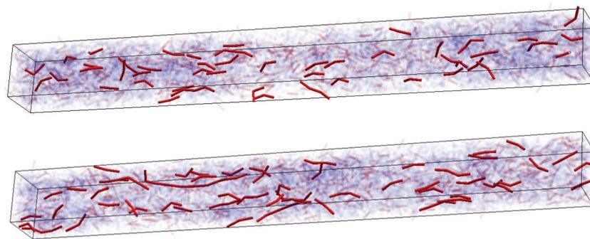
**Fig. 8** Distribution of stretched segments (red cylinders) in resultant gels for s2020 (top) and Rnd (bottom) under the applied stretch  $\lambda = 5$ . The stretched segments are highlighted when consecutive segments are stretched. For the colored segments, the squared segment length is larger than 3. The dispersed beads are also shown by light blue spheres.
