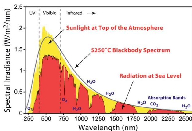
Fig. 1 The air mass (AM) 1.5 solar spectrum [https://commons.wikimedia.org/wiki/File:Solar\_spectrum\_en.svg].
