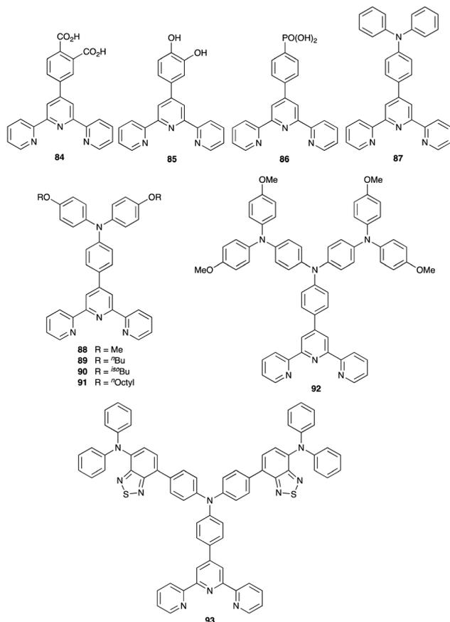
Scheme 28 Structures of derivatives of tpy used as anchoring (84–86) and ancillary (87–93) ligands in zinc(II) dyes.
