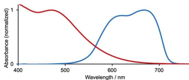
Fig. 10 Solid-state absorption spectra of FTO/TiO<sub>2</sub> electrodes with adsorbed dyes  $[Cu(11)(45)]^+$  (red) and SQ2 (blue). The high-energy tail arises from TiO<sub>2</sub> absorption (spectra recorded by Frederik Malzner, University of Basel).
