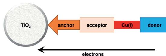
Fig. 8 A schematic representation of structural design for a heteroleptic bis(diimine)copper(i) sensitizer facilitating electron transfer through the dye molecule to the n-type semiconductor.
