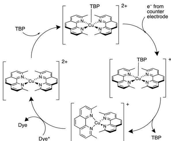
Scheme 7 Representation of the involvement of a strong Lewis base such as TBP in the redox cycle of the  $[\text{Cu}(\text{Me}_2\text{phen})_2]^{2+}/[\text{Cu}(\text{Me}_2\text{phen})_2]^+$  mediator. Based on a scheme from the work of Bach and coworkers.<sup>119</sup>
