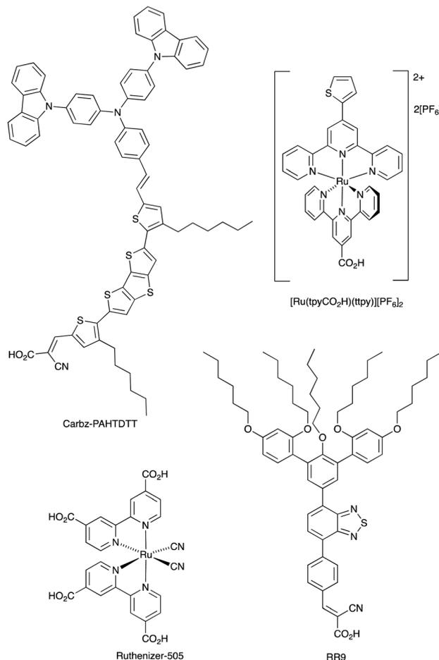
Scheme 12 Structures of the metal-free dyes Carbz-PAHTDIT and RR9, and the ruthenium(II) dyes [Ru(tpyCO<sub>2</sub>H)(tppy)][PF<sub>6</sub>]<sub>2</sub> (tpy = 2,2':6',2''-terpyridine) and the commercially available Ruthenizer-505.
