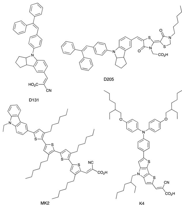
Scheme 11 Structures of the commercially available dyes D131 and D205, and of the metal-free dyes MK2 and K4.
