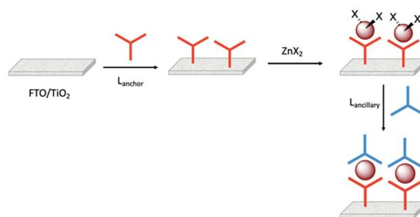
Fig. 15 The SALSAC approach to *in situ* assembly of a heteroleptic bis(terpyridine)zinc(II) dye on an electrode surface using a stepwise strategy.  $\text{ZnX}_2$  is typically  $\text{Zn}(\text{OAc})_2$  or  $\text{ZnCl}_2$ .
