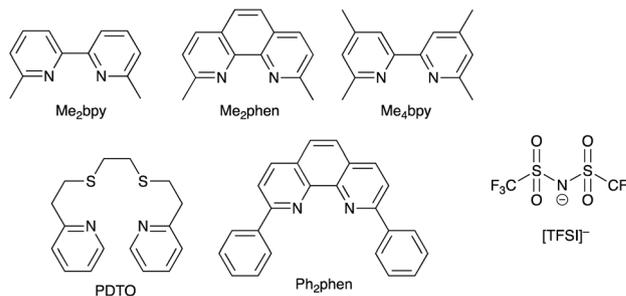
Scheme 6 Structures of some of N^N ligands used in copper(II)/copper(I) redox mediators, and the structure of the [TFSI]<sup>-</sup> anion.
