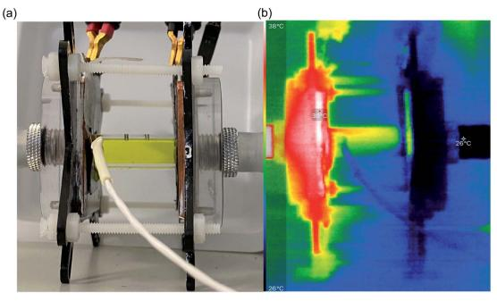
Fig. 4 Photos of (a) the actual thermogalvanic cell, sandwiched between the two heat exchangers (the white wire coming from the left is the heat flux sensor wiring); electrode separation = 29.3 mm,  $\Delta T_{app} = 20$  K; and (b) IR image of the same cell, going from white = hottest to black =
