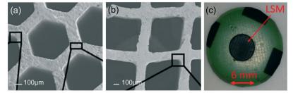
Fig. 22 (a) Hexagonal, and (b) square CGO microstructures of 12 μm depth each, comprising 20 printed layers. Reproduced with permission.<sup>88</sup> (c) photograph of the printed LSM deposited using aqueous-based ink.
