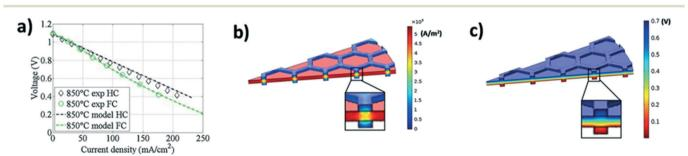
Fig. 7 (a) Predicted effect of inkjet-printed 3D honeycomb structure on the power generation performance calculated through a simulation (dashed lines); (b) current and (c) voltage distributions throughout the 3D printed structure calculated by the numerical simulation (reproduced with permission<sup>36</sup>).
