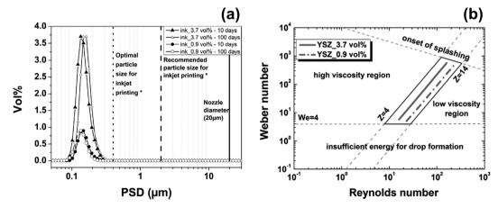
Fig. 15 (a) Particle size distributions for 3.7 vol% and 0.9 vol% YSZ ink after milling for 10 days and after 100 days of storage (b) Weber-Reynolds numbers diagram defining the printability conditions for those YSZ inks. 80
