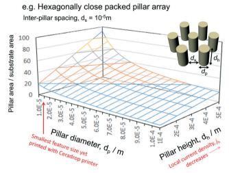
Fig. 6 Effect on pillar area/substrate area of pillar diameter and height of hexagonally close packed pillar array on planar substrate.
