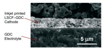
Fig. 21 SEM image of the cross section of the printed cathode layer. Reproduced with permission.87
