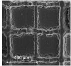
Fig. 18 (a) 50 and (b) 180 layers of YSZ printed to fabricate micro-pillar arrays; (c) a YSZ square lattice printed onto a NiO-YSZ substrate. Reproduced with permission.<sup>31</sup>
