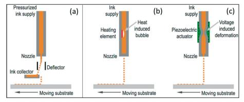
Fig. 3 Schematic representation of (a) continuous inkjet (CIJ) and drop on demand (DOD) inkjet printing systems using (b) thermal and (c) piezoelectric technology (reproduced with permission<sup>33</sup>).
