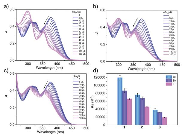
Fig. 4 (a-c) UV-vis spectra of metallacycle 1 with increasing concentrations of TBACI, TBABr and TBAI in  $CH_3CN$ . (d) Binding constants ( $K_a$ ) of metallacycles 1-3 with TBACI, TBABr and TBAI.
