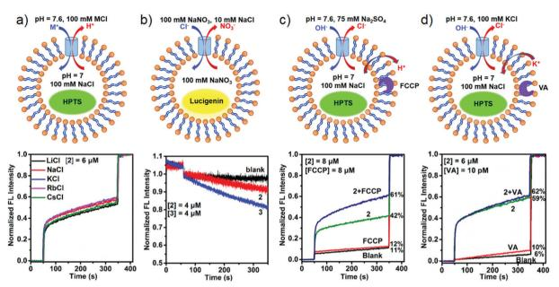
Fig. 6 (a) Cation selectivity evaluated by the HPTS assay. (b) Lucigenin assay using a chloride-sensitive lucigenin dye. (c) Comparison of the ion transport activity of 2 in the presence and the absence of FCCP. (d) Comparison of the ion transport activity of 2 in the presence and the absence of VA.
