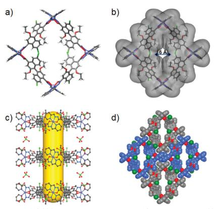
Fig. 2 (a) Single-crystal X-ray structure of 2. (b) Solvent-accessible iso-surface model of 2 shown from the above. (c) Packing of 2 to generate a nanotube. (d) The extended structures are generated with four rings. Gray: C; red: O; green: Cl; white: H; dodger blue: N; light blue: Zn. The channel is highlighted by the yellow stick.
