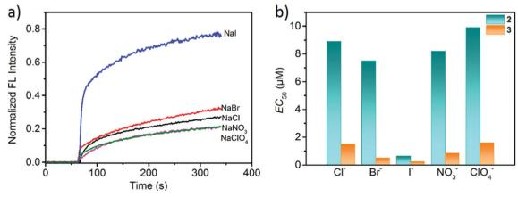
Fig. 8 (a) Transport activities toward Cl<sup>-</sup>, Br<sup>-</sup>, I<sup>-</sup>, NO<sub>3</sub><sup>-</sup> and ClO<sub>4</sub><sup>-</sup> at a final concentration of  $1\,\mu\text{M}$  for **2** (**2**: lipid = 1:375). The background rates of I<sup>-</sup> and  $ClO_4^-$  were subtracted. (b) The  $EC_{50}$  values for **2** and **3** mediated transport of  $Cl^-$ ,  $Br^-$ ,  $I^-$ ,  $NO_3^-$  and  $ClO_4^-$  determined using the HPTS assay.
