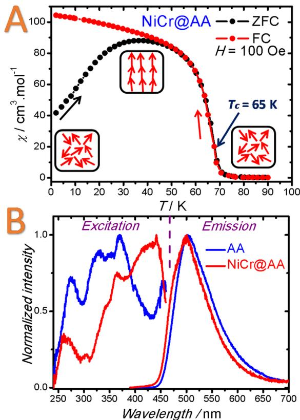
**Fig. 9** (A) Zero Field Cooled (ZFC)/Field Cooled (FC) curves performed for NiCr@AA with an applied magnetic field of 100 Oe and showing the Curie temperature ( $T_c$ ) at 65 K; (B) room temperature excitation and emission spectra for NiCr@AA. Reproduced from ref. 223 with permission from the Royal Society of Chemistry.
