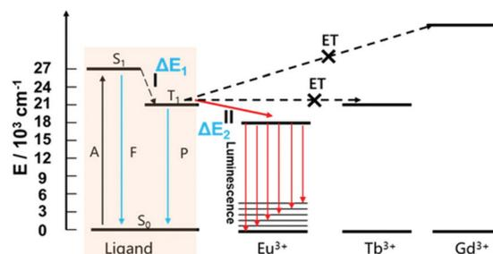
Fig. 3 The luminescence mechanism of the Eu-MOF (A: absorption; F: fluorescence; P: phosphorescence; I: intersystem crossing; II: energy transfer between T<sub>1</sub> of ligand and  $^5D_0$  of Eu<sup>3+</sup>).
