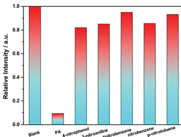
**Fig. 7** Luminescence responses of the Eu-MOF in various nitro explosives (0.1 mM) in DMAC.
