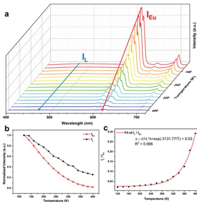
**Fig. 4** (a) Emission spectra ( $\lambda_{\text{ex}} = 365 \text{ nm}$ ) of the Eu-MOF in the temperature range of 120–400 K (b) The changing trend of the luminescence intensity ( $I_{\text{ligand}}$  and  $I_{\text{Eu}}$ ). (c) The measured temperature parameters ( $\Delta = I_L/I_{\text{Eu}}$ ) and the fitted line by Boltzmann law.
