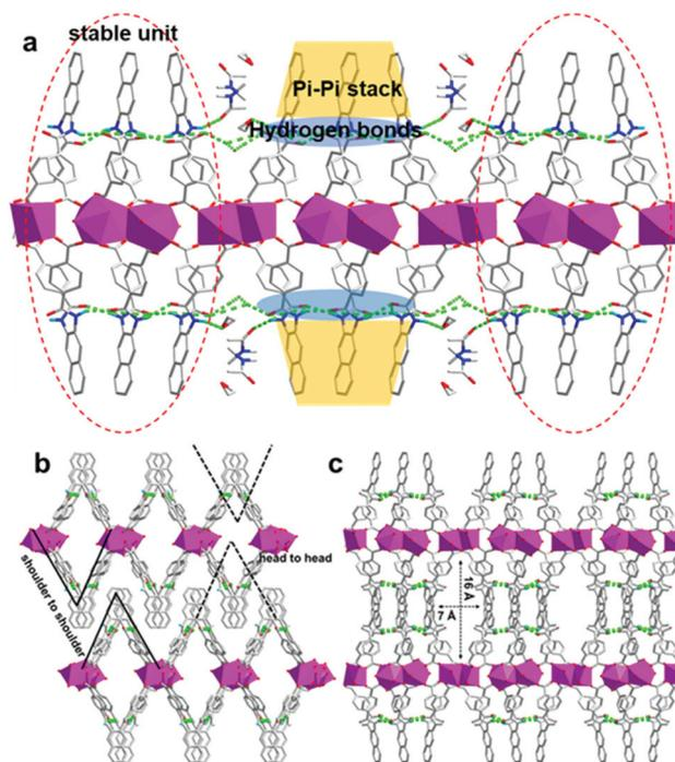
**Fig. 2** (a) Hydrogen bonding interactions and  $\pi$ – $\pi$  stacking interactions every layer. (b) The stack way of layers. (c) 3D structure viewing along  $c$  axis.
