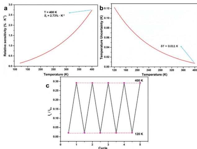
**Fig. 5** (a) The relative sensitivity ( $S_r$ ) of the Eu-MOF. (b) The temperature uncertainty ( $\delta T$ ) of the Eu-MOF. (c) The reversible emission intensity ratio ( $I_L/I_{Ln}$ ) of the Eu-MOF between 120 K and 400 K.
