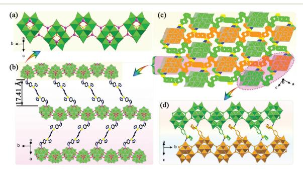
Fig. 2 Structure of compound 2: (a) the 1D zigzag inorganic chain; (b) the 2D grid-like layer; and (c and d) the 3D covalent framework. Color code: W, green; {WO<sub>6</sub>} octahedron or simplified 1D chain, green or orange; Zn, pink; K, yellow; O, red; N, blue; C, black.
