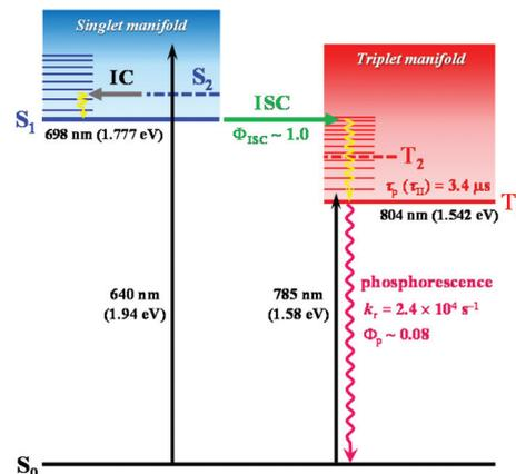
**Fig. 4** Excited state deactivation pathway and related photophysical parameters for the Au<sub>25</sub>-rod in deaerated THF. The vertical transition energy from  $S_0$  to  $S_1$  or  $T_1$  obtained from theoretical calculations is also shown. The  $S_2$  and  $T_2$  states theoretically predicted to exist in the energetic vicinity of the  $S_1$  and  $T_1$  states (Fig. S11†) are shown as dashed lines.
