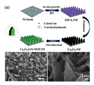
**Fig. 3** (a) Schematic illustration of the preparation of Co<sub>3</sub>O<sub>4</sub>@Ni-MOF/NF. (b and c) SEM images of the as-prepared Co<sub>3</sub>O<sub>4</sub>@Ni-MOF/NF. Reprinted with permission from ref. 57, Copyright 2021, Royal Society of Chemistry.
