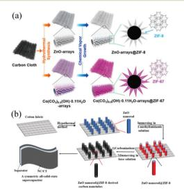
Fig. 5 (a) Scheme showing the synthetic process of ZnO@ZIF-8 and Co (CO $_3$ )0.5(OH)·0.11H $_2$ O@ZIF-67 on CC. Reprinted with permission from ref. 63, Copyright 2018, American Chemical Society. (b) Schematic illustration showing the fabrication of ZnO@ZIF-8 derived nanotubes. Reprinted with permission from ref. 64, Copyright 2018, Elsevier.
