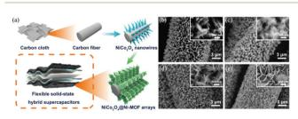
Fig. 4 (a) Schematic illustration of the synthesis of  $NiCo_2O_4@Ni-MOF$  on CF. (b–e) SEM images of  $NiCo_2O_4@Ni-MOF$  synthesized at 3, 6, 12, and 24 h for MOF growth, respectively. Reprinted with permission from ref. 58, Copyright 2019, American Chemical Society.
