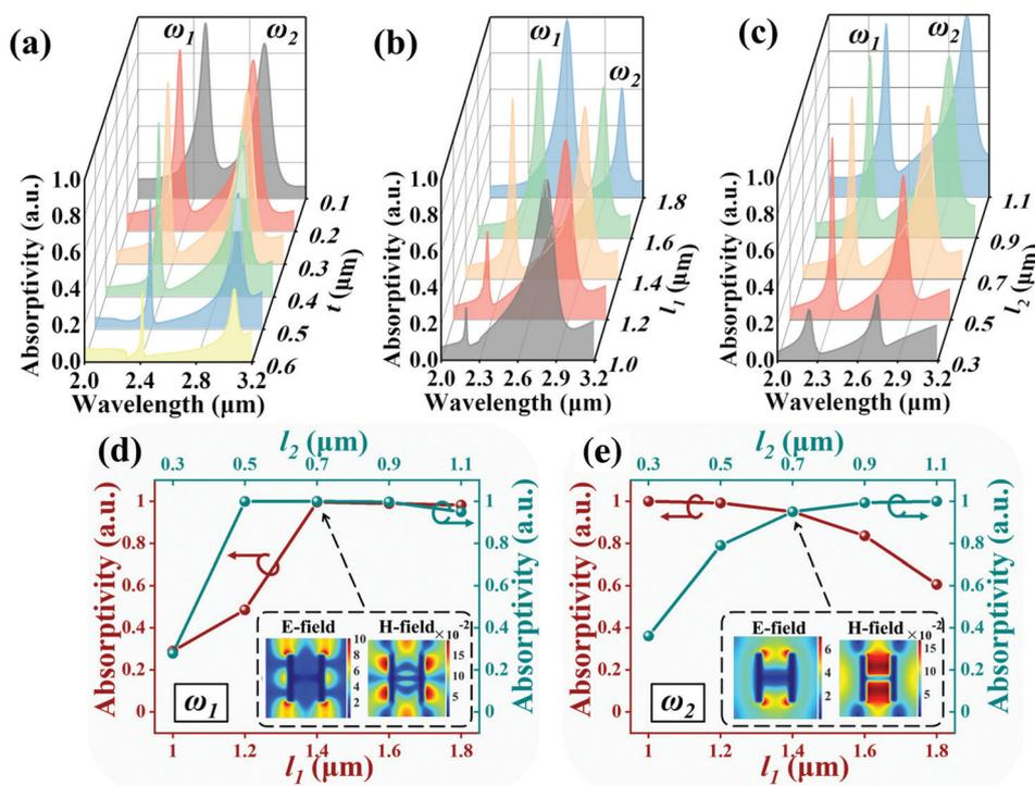
**Fig. 2** Absorptivity of the H-shaped MPA with different (a)  $t$ , (b)  $l_1$ , and (c)  $l_2$  values, respectively. The relationships of the resonance intensities of the H-shaped MPA with different  $l_1$  and  $l_2$  values at (d)  $\omega_1$  and (e)  $\omega_2$  resonances, respectively. The inserted images show the corresponding  $E$ -field and  $H$ -field distributions under the conditions of  $l_1 = 1.4 \mu\text{m}$  and  $l_2 = 0.7 \mu\text{m}$ .
