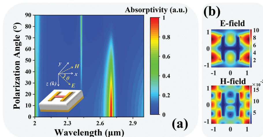
Fig. 3 (a) Absorptivity of the H-shaped MPA at different polarization angles. (b) The corresponding  $E$ -field and  $H$ -field distributions with a polarization angle of 90° at a wavelength of 2.40  $\mu\text{m}$ .
