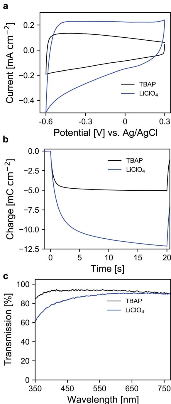
Fig. 2 (a) CVs of ATO (2% Sb) mesoporous electrode layers measured in TBAP/PC and LiClO<sub>4</sub>/PC with a scan rate of 20 mV s<sup>-1</sup>. (b) Coulometric measurement for a potential step between +0.3 V and -0.6 V vs. Ag/AgCl in both electrolytes. (c) UV/VIS transmission spectra of ATO electrodes (after negative polarization) without an applied potential for both electrolytes; optical reference: an electrolyte-filled cell with blank FTO glass.
