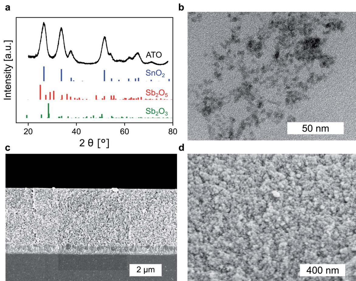
Fig. 1 (a) XRD of ATO nanoparticles (2% Sb) along with the reference spectra of  $\text{SnO}_2$  (ICSD: 39177, blue),  $\text{Sb}_2\text{O}_5$  (ICSD: 8050, red) and  $\text{Sb}_2\text{O}_3$  (ICSD: 2033, green). (b) TEM image of ATO nanoparticles after autoclave treatment. (c) Cross-sectional SEM of ATO layers on FTO. (d) Magnified cross-sectional view displaying the mesoporous structure of the nanoparticle layers.
