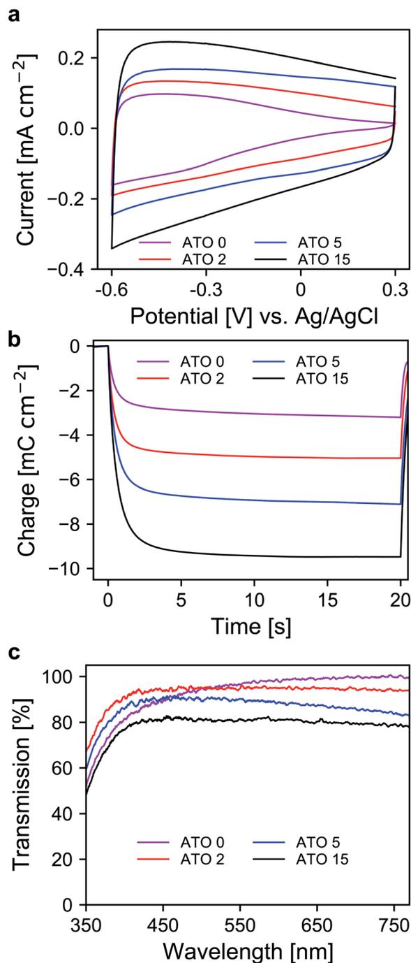
Fig. 3 (a) CVs of ATO mesoporous electrode layers with different antimony doping levels measured in TBAP/PC with a scan rate of  $20 \text{ mV s}^{-1}$ . (b) Coulometric measurement for a potential step between  $+0.3 \text{ V}$  and  $-0.6 \text{ V}$  vs. Ag/AgCl. (c) UV/VIS transmission spectra of ATO electrodes at  $+0.3 \text{ V}$  vs. Ag/AgCl; optical reference: an electrolyte-filled cell with blank FTO glass.
