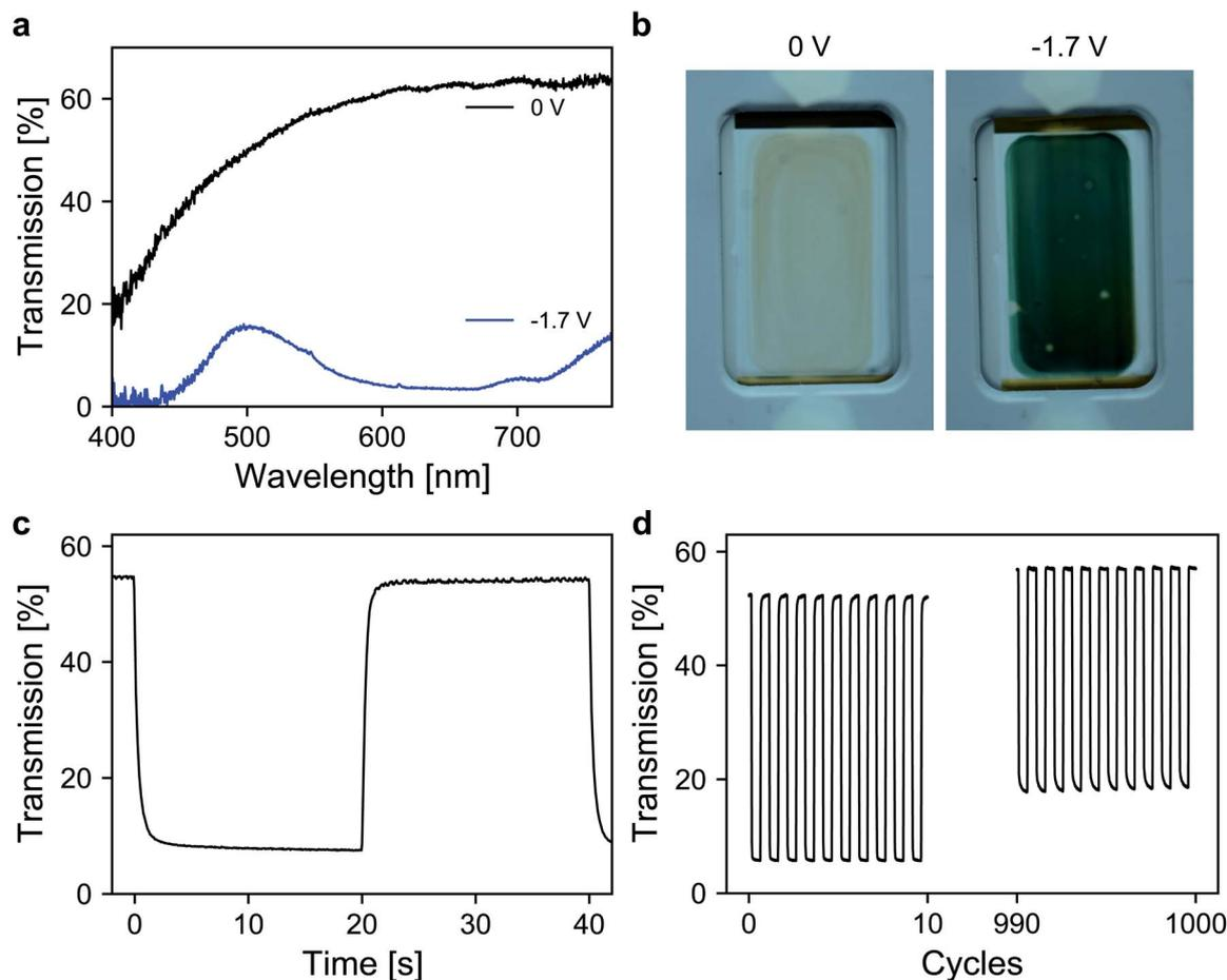
Fig. 5 (a) Transmission spectra of the device at 0 V and  $-1.7$  V. (b) Images of the device in the bleached (left) and colored (right) states. (c) Time depended transmission change for one switching cycle. (d) Transmission change over 1000 (e)coloration cycles.
